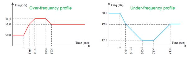
Figure 1 Overfrequency and underfrequency withstanding capabilities
