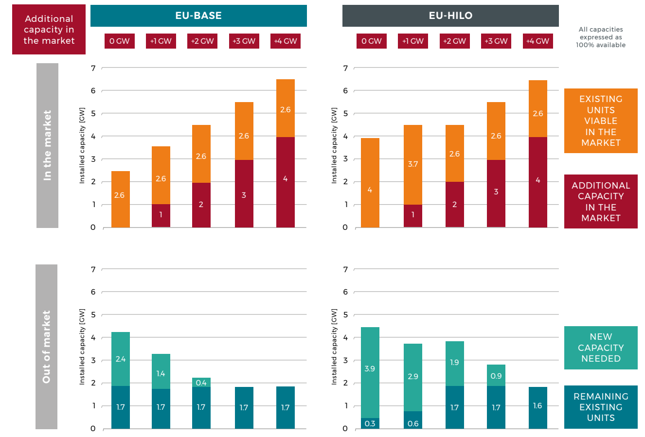
ECONOMIC VIABILITY CHECK OF EXISTING AND NEW CAPACITY WHEN ADDING CAPACITY TO THE BELGIAN MARKET (WITH MARGINAL PRICE LOWER OR EQUAL TO AN EFFICIENT CCGT) FOR 2025 [FIGURE 4-17]
