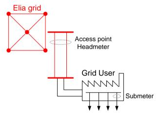
TSO Submetering Delivery Points will be measured by a Submetering facility.
