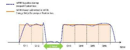
Figure 1 - Prequalification test to apply for mFRR Standard only
