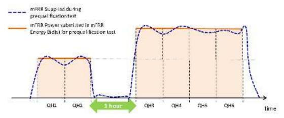
Figure 3 – Prequalification test to apply for mFRR Standard and mFRR Flex
