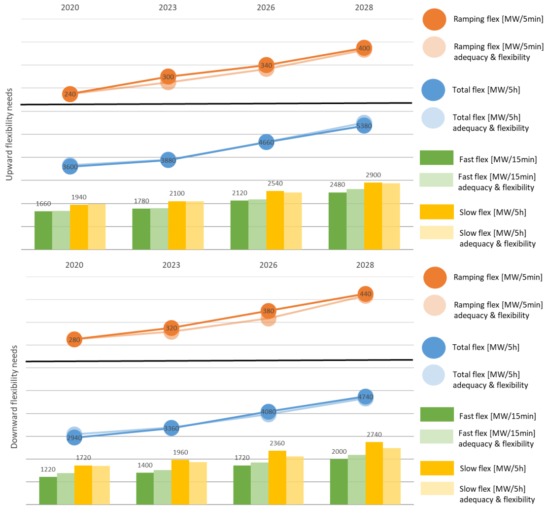
Figure 19: upward (up) and downward (down) flexibility needs in the H-RES scenario toward 2028 (expressed in MW)
