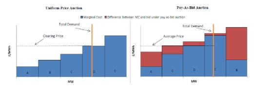
Figure 2: Non-optimal dispatch in case of paid-as-bid, compared to paid-as-cleared<sup>6</sup>
