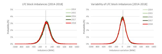
Figure 8: Probability distribution of the LFC block imbalances between 2014 and 2018 (in steps of 10 MW)
