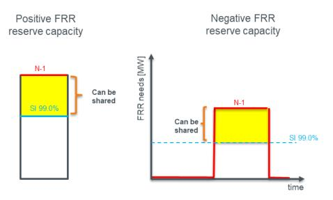
Figure 11: Visual representation of the maximal sharing potential following SOGL by the surface between dimensioning incident (N-1) and historic LFC-block imbalances (SI 99%) for dimensioning positive FRR needs (left) and negative FRR needs (right)
