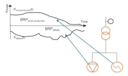
Figure 3: Allocations of energy according to annex 3bis: the BRP responsible for the load is being attributed all offtake metered at asset level whereas the BRP responsible for the local production unit(s) is being attributed all metered volume injected (metered at asset level) by the local production unit(s) (non-netted)
