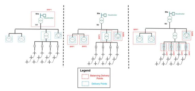
Figure 12: Three different examples of possible configurations of BDPs and DPs
