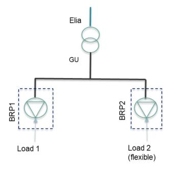
Figure 2: Example of a possible configuration where a separate  $BRP_{source}$  is designated only for the asset providing flexibility
