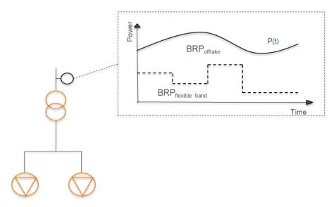
Figure 7: Allocations of energy according to annex 11. The energy is metered at the Access Point level. A changing part of it is allocated to  $BRP_{flexible\ band}$  and the rest is allocated to  $BRP_{offtake}$ .
