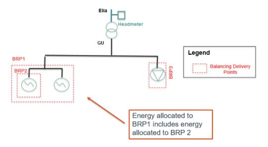
Figure 10: Not allowed configuration due to overlap of BDPs perimeter
