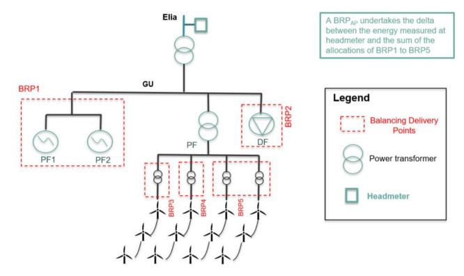
Figure 9: Schematic example of the proposed multi-BRP design. To be noted that for the different strings of wind turbines the anchoring is at metering points, not transformers.
