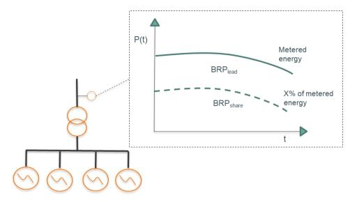
Figure 5: Allocations of energy according to annex 9. The energy is metered at the Access Point and a percentage of it is attributed to different BRPs according to a fixed key.
