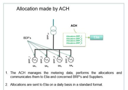
Figure 11: Allocation communication to be made by ACH's
