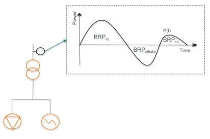
Figure 4: Allocations of energy according to annex 3ter: the BRP responsible for offtake is being attributed the net offtake metered at the Access Point whereas the BRP responsible for injection is being attributed the net injection metered at the Access Point
