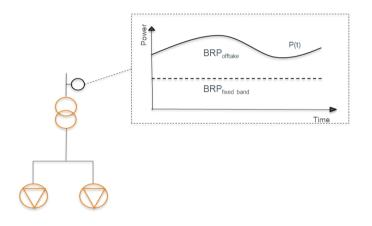
Figure 6: Allocations of energy according to annex 10. Energy is measured at the Access Point. A fixed part of it is allocated to the BRP<sub>fixed band</sub> and the rest is allocated to the BRP<sub>offtake</sub>
