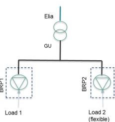
Figure 2: Example of a possible configuration where a separate BRP<sub>source</sub> is designated only for the asset providing flexibility
