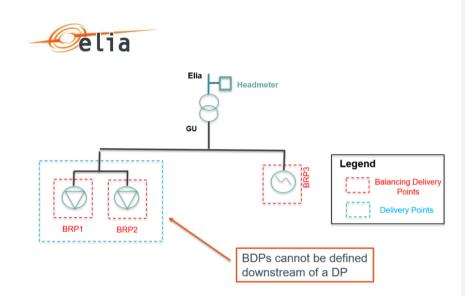
Figure 13: Example of a non-possible configuration of BDPs and DPs
