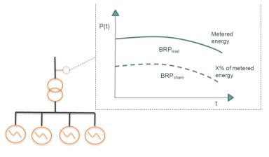
Figure 5: Allocations of energy according to annex 9. The energy is metered at the Access Point and a percentage of it is attributed to different BRP'sBRPs according to a fixed key.
