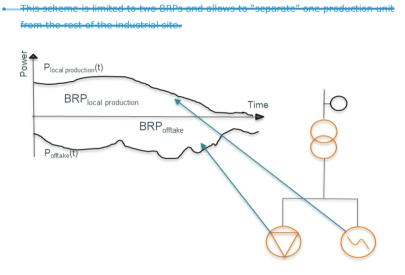
Figure 3: Allocations of energy according to annex 3bis: the BRP responsible for the load is being attributed all offtake metered at asset level whereas the BRP responsible for the local production unit(s) is being attributed all metered volume injected (metered at asset level) by the local production unit(s) (non-netted)
