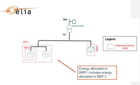
Figure 10: Not allowed configuration due to overlap of BDPs perimeter
