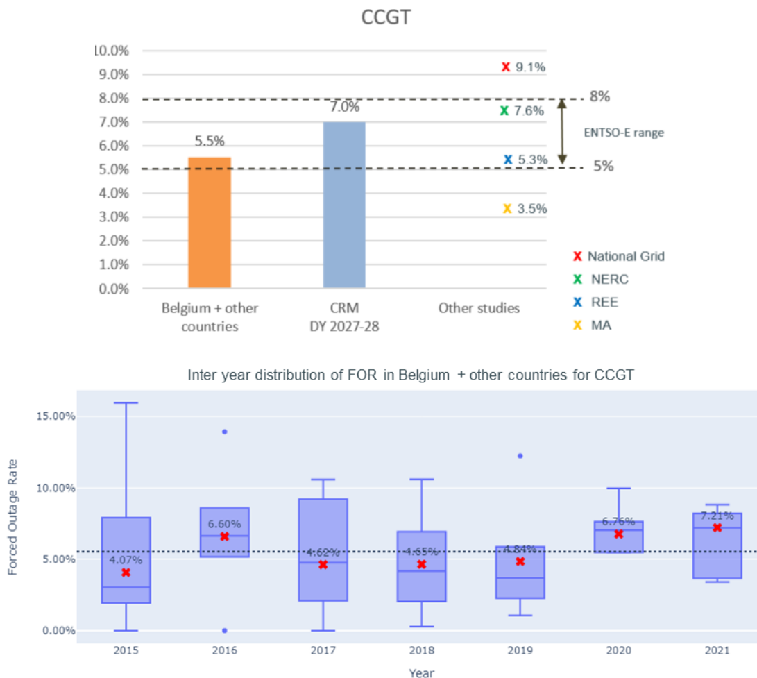
Figure 3: Forced outage rates for CCGT – Detailed analysis
