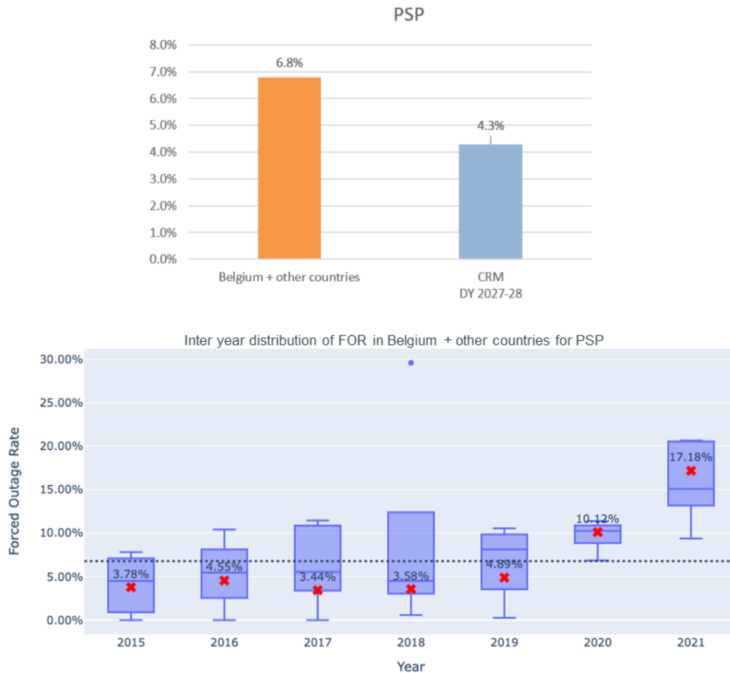
Figure 6: Forced outage rates for PSP – Detailed analysis
