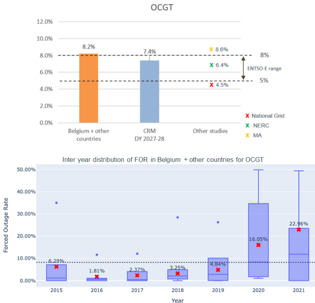
Figure 4: Forced outage rates for OCGT – Detailed analysis
