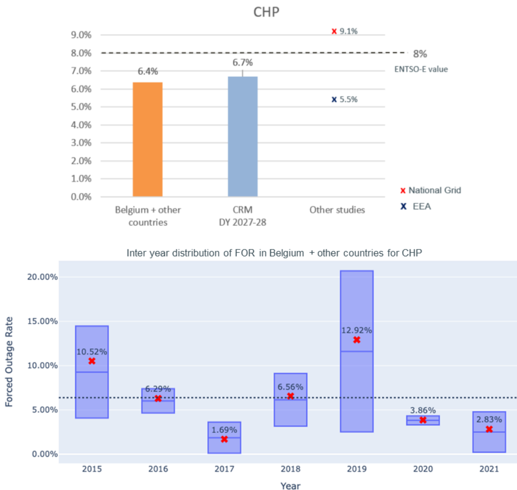
Figure 5: Forced outage rates for CHP – Detailed analysis
