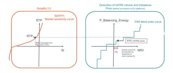
'RTP3' being different from 'RTP2' a third iteration of the loop occurs, leading to a volume 'x3' to be activated explicitly and hence to a real-time price 'RTP4' which, this time, is equal to 'RTP3'.
