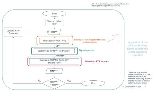
Figure 21 – Example of smart balancing controller implementation
