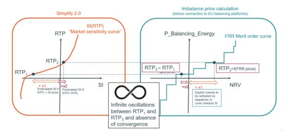
If the loop was not broken with additional conditions (for instance based on the maximum number of iterations), this situation would create infinite oscillations between 'RTP1' and 'RTP3' and no convergence would be reached.
