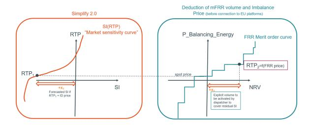
Since 'RTP2' and 'RTP1' are different, the smart balancing controller loop has not converged yet, and the loop is entered again with a new RTP value, for instance equal to 'RTP2'.
