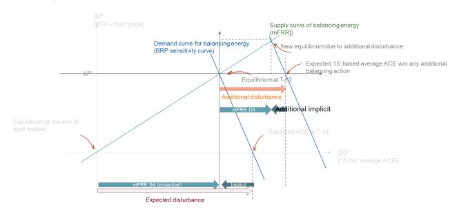
Figure 19 – Deviation from the last real-time equilibrium (calculated at T-13) due to forecast errors/additional disturbance
