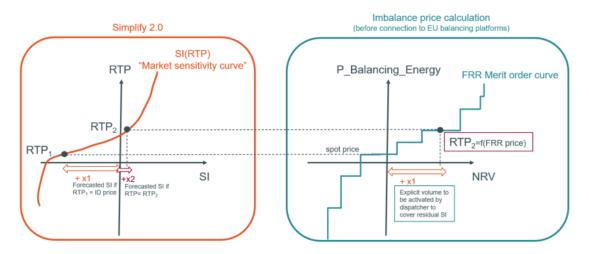
This residual system imbalance is covered by explicit activations of downward bids offered at the price of the last market equilibrium ('spot price'), resulting in a new RTP which is again equal to 'RTP1'.
