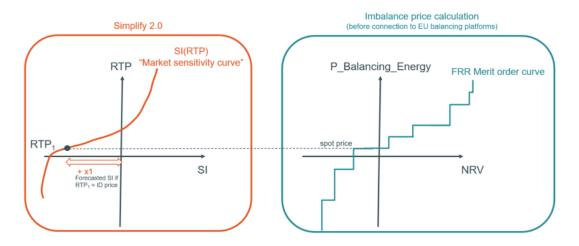
This system imbalance needs to be entirely covered by explicit activations, leading to a new RTP equal to 'RTP2'.
