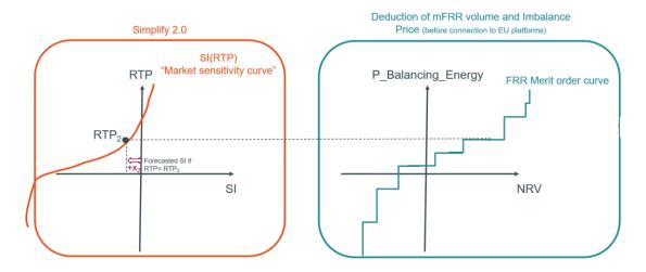
Again, this forecasted residual system imbalance 'x2' needs to be exclusively covered by FRR activations, leading to a new RTP equal to 'RTP3'.
