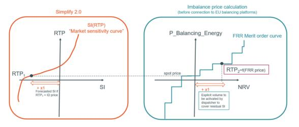
This new RTP being higher than the price of the last market equilibrium, it stimulates an implicit reaction that makes the system slightly switch in the other direction, leading to a positive residual system imbalance 'x2'.
