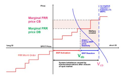
Figure 12 – Illustration of the loss of social welfare in a central balancing model
