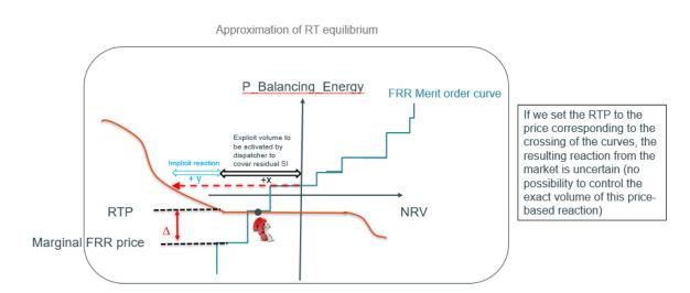
At that moment, an efficient way to balance the system could (for instance) consist in limiting the RTP to a price that does not stimulate the large amount of flexibility reacting to the same price signal, and to cover the residual imbalance by activating more explicit flexibility for which the operator has perfect control on the volume. This, again, creates a slight deviation of the real-time price from the marginal price of the activated FRR bids. This possible
