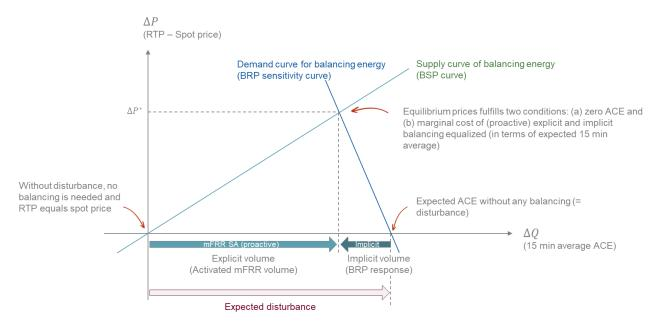
Figure 18 - most efficient real-time equilibrium calculated at T-13, defining the mFRR volume to be activated in SA and the RTP forecast
