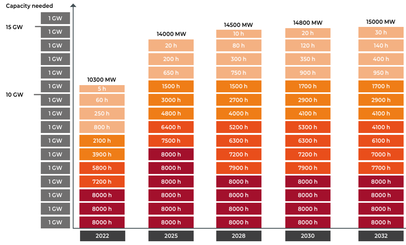
[FIGURE 5-3] — RESIDUAL LOAD FOR BELGIUM; DURING HOW MANY HOURS IS A CERTAIN CAPACITY REQUIRED, IN ADDITION TO RES AND NUCLEAR CAPACITY ACCORDING TO 'CENTRAL' SCENARIO ?
