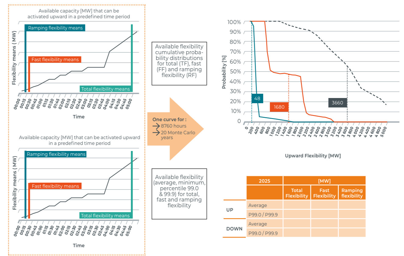
[FIGURE 4-34] — ILLUSTRATION OF THE AGGREGATION OF AVAILABLE FLEXIBILITY (LEFT) AND INDICATORS TO ASSESS AVAILABLE FLEXIBILITY PER TYPE (RIGHT)
