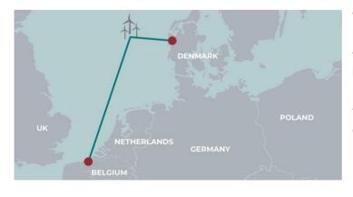
When the interconnector between Belgium and Denmark is completed, the cable will run through the territorial waters of four countries: Belgium, the Netherlands, Germany and Denmark. Stretching over 600 km, it could be the longest subsea direct-current (HVDC) cable in the world.
