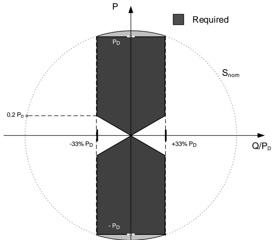
Figure 3: Capability curve for SPM type B
