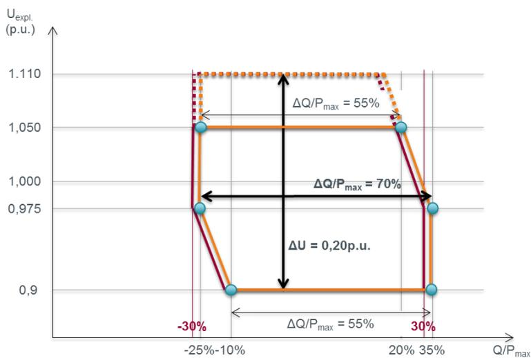
Figure 7 U-Q/P<sub>max</sub> profile for a type C and D SPM (dashed for nominal voltages above 300kV).
