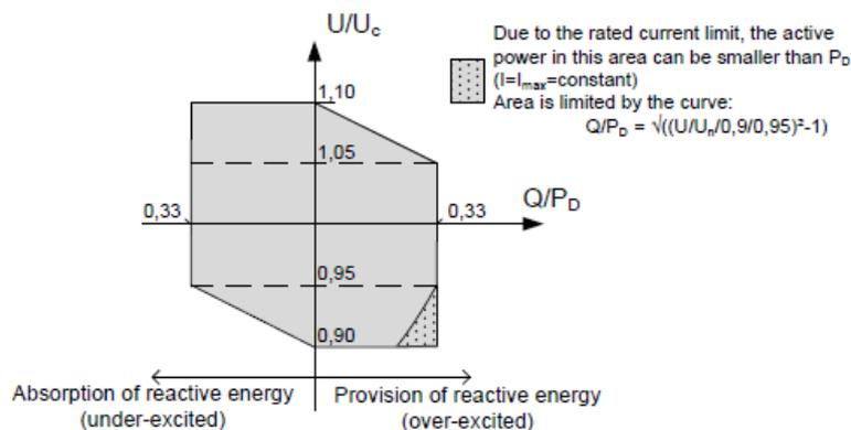
Figure 4: U-Q/P<sub>D</sub> profile for type B SPM in order to visualize reactive power requirements for voltages different from 1pu.
