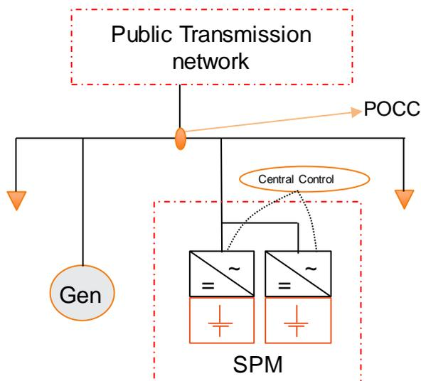
Figure 1 Example of Storage Park Module grid connection
