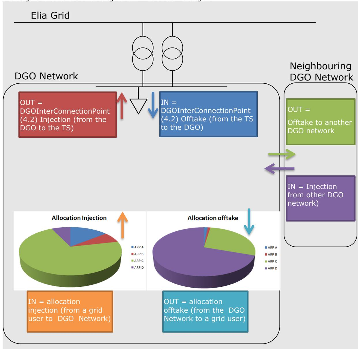
Figure 11: DGO Loop losses (DGO PBO) directions
