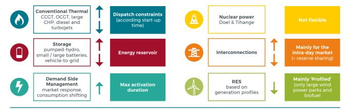
Firstly, the ability to provide flexibility is determined by the **operational characteristics** (minimum up/down time, hot/warm/cold start-up time, transition time from hot to warm / warm to cold, minimum stable power, rated power and the ramp rate). In general, these constraints are particularly relevant for thermal power plants.
