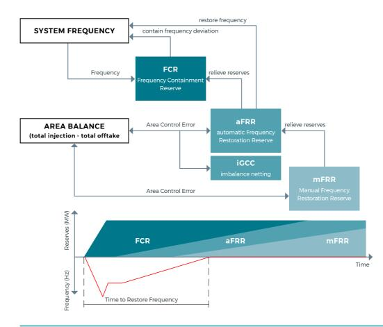
The Frequency Restoration Reserve (FRR) must free up the FCR of the synchronous zone to prevent network instability, or even a failure of the entire electricity system, in the event of additional system imbalances. Each control area is therefore obliged to maintain its balance which is monitored by means of quality criteria assessing the Area Control Error (ACE), i.e. the real-time deviation between measured and scheduled cross-border exchanges on a quarter-hourly (and even by minute) basis.
