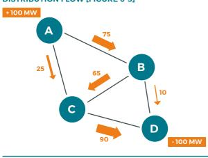
Let's assume the simplified grid example on Figure 6-3. If an exchange from Node A to Node D of 100 MW occurs, the PTDF factors could be:
