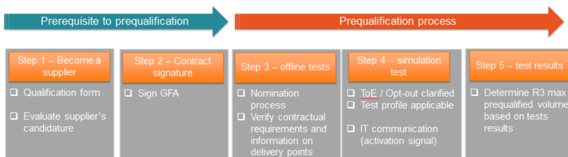
Figure 6 : overview of the prequalification process applicable to both R3 down CIPU and R3 down non CIPU contracts
