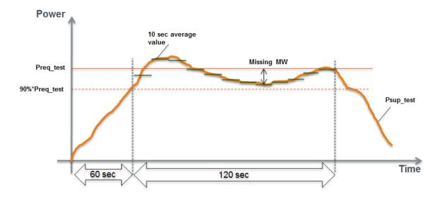
If the  $P_{sup\_test}(t)$  value drops below the level of 90% of  $P_{req\_test}(i)$  at any time during the test's delivery timeframe(s), ELIA will calculate the  $Av\_P_{sup\_test}(i)$  values (as figuring in the above formula) using <u>exclusively</u> the  $P_{sup\_test}$  values that are lower than 90% of  $P_{req\_test}(i)$ .
