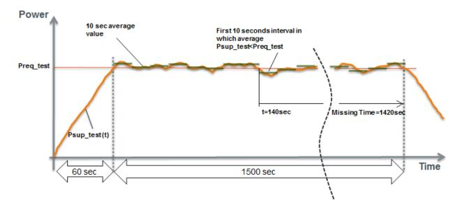
In the example displayed hereby above, the 10-seconds average value of  $P_{\text{sup\_test}}(t)$  becomes inferior to  $P_{\text{req\_test}}(i)$  for the first time at the interval starting at t=140 sec.
