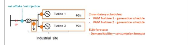
The schedule gives a value in MW for each quarter-hour of day D representing the average generated power during the concerned quarter-hour, regardless of whether the Power Generating Module feeds a local offtake or directly injects onto the electricity grid.
