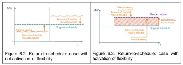
If the schedule had been amended by ELIA following the activation of flexibility for redispatching or balancing, the return-to-schedule principle equally applies in both directions with the new schedule as baseline. Figure 6.3 shows the case of an incremental activation of flexibility.
