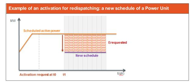
In the case of a decremental activation on a Power Unit (as in the example), the new schedule represents a maximum power output. The **implications** are the following:
