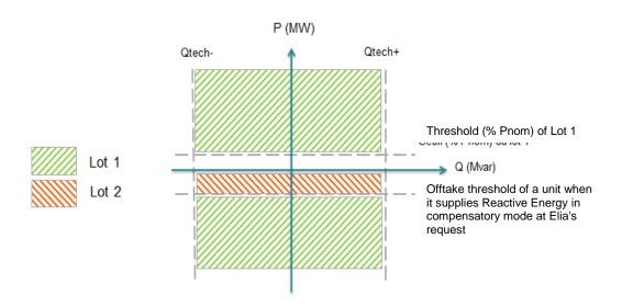
The Reactive Power generated or absorbed by a Production Unit referred to in the Contract is the Reactive Power measured by Elia at the Injection Point, i.e. on the high-voltage side of the step-up transformer of that Production Unit.
