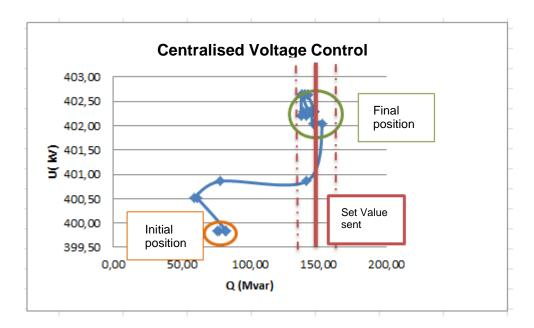
For instance, if the set value communicated by Elia for this example had been 200 Mvar, Elia would have noted in its measurements that the maximum value attained by the unit is 152.86 Mvar.
