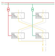
Moreover, the grid user may install additional crosschecks to avoid unwanted tripping of his feeders, provided the total tripping time can be respected. For example, the grid user may install a device which blocks the disconnection of the load if the there is no frequency drop.
