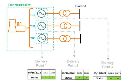
The figure below illustrates the case of a wind park which is a Power Park Module (PPM) whose primary energy source is wind. The delivery point for the provision of the availability statuses is defined at the level of the technical unit (which is by default also the technical facility as it is a PPM)
