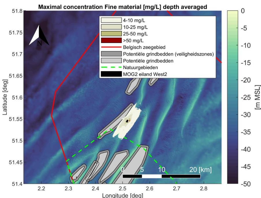
Figure 4-28 Maximal encountered depth averaged sediment concentration [mg/L] of fine material (< 250 [µm]) during the simulation period. Scenario: Plume generation and deposition as a result of natural erosion in one year time after West 2 island construction, after four year case.
