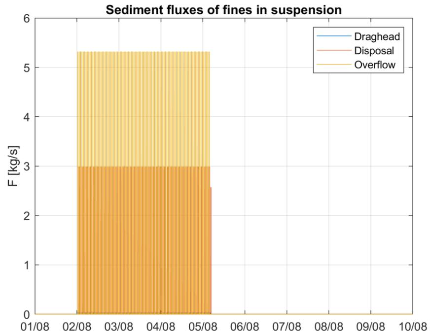
Figure 7-5 Time series of the implemented source of fines ( $d_p < 63 \mu\text{m}$ ) [kg/s] as a result of pre-dredging scour holes and ridges and disposing dredged material at the island location at the Noord location.
