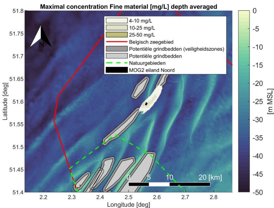
Figure 4-32 Maximal encountered depth averaged sediment concentration [mg/L] of fine material (< 250 [μm]) during the simulation period. Scenario: Plume generation and deposition as a result of natural erosion in one year time after Noord island construction, after four year case.
