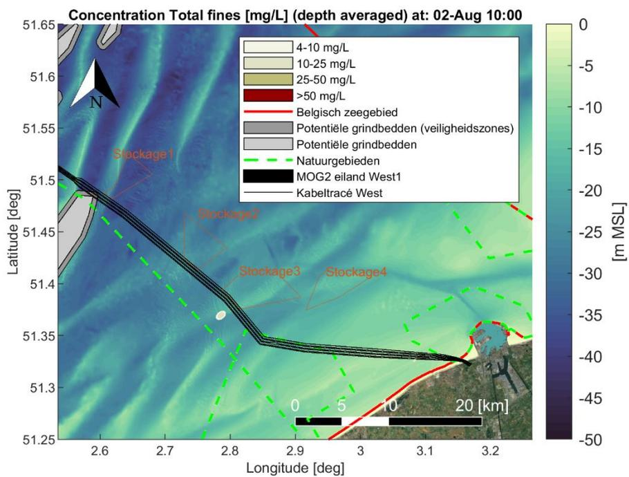
Figure Annex B-21 Map showing encountered depth averaged sediment concentration [mg/L] of fine material (< 250 [µm]) during a time instant of the simulation period. Scenario: Dredging cable trenches (trench1 section) and disposal at a temporary disposal site (Stockage3).
