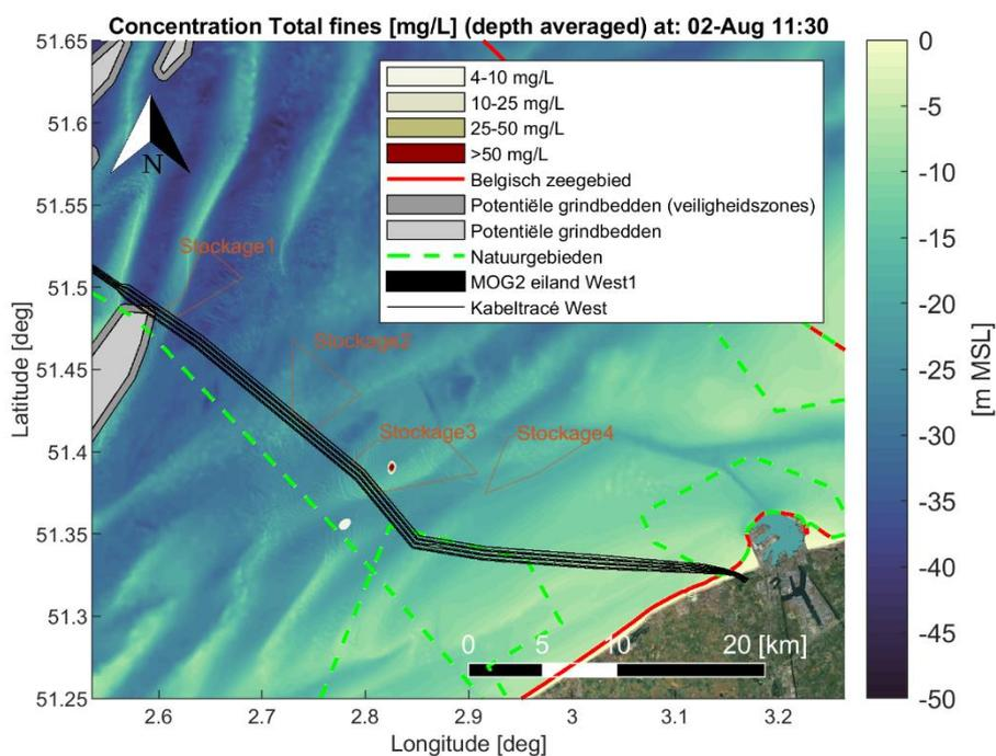
Figure Annex B-24 Map showing encountered depth averaged sediment concentration [mg/L] of fine material (< 250  $\mu\text{m}$ ) during a time instant of the simulation period. Scenario: Dredging cable trenches (trench1 section) and disposal at a temporary disposal site (Stockage3).
