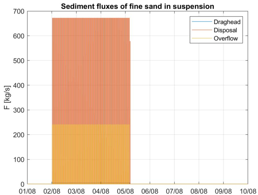
Figure 7-6 Timeseries of the implemented source of fine sand [kg/s] as a result of pre-dredging scour holes and ridges and disposing dredged material at the island location at the Noord location.
