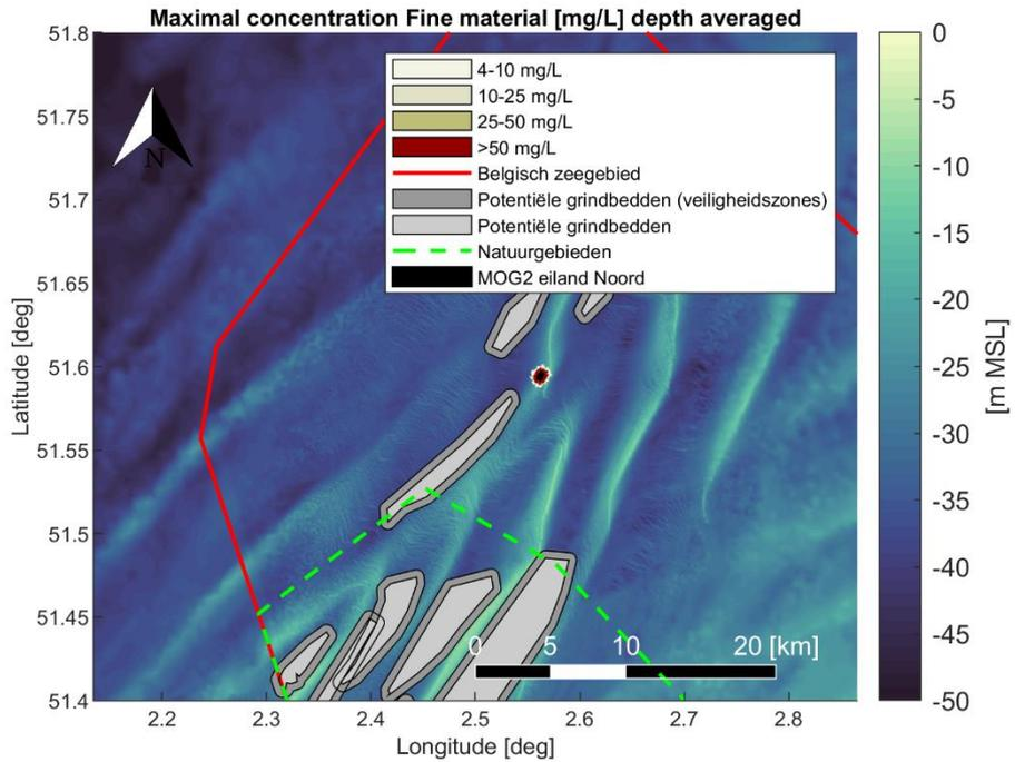
Figure 4-11 Maximal encountered depth averaged sediment concentration [mg/L] of fine material ( $< 250 [\mu m]$ ) during the simulation period. Scenario 3: pre-dredging scour holes and filling the Noord island ring.
