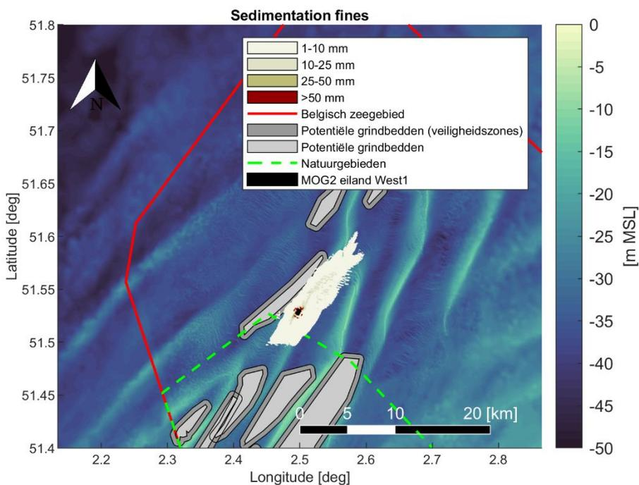
Figure 4-21 Maximal sedimentation [mm] of fine material (< 250 [μm]) during the simulation period. Scenario: Plume generation and deposition as a result of natural erosion in one year time after West 1 island construction, after one year case.
