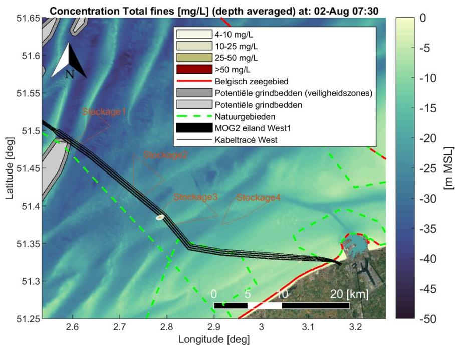
Figure Annex B-16 Map showing encountered depth averaged sediment concentration [mg/L] of fine material (< 250 [μm]) during a time instant of the simulation period. Scenario: Dredging cable trenches (trench1 section) and disposal at a temporary disposal site (Stockage3).
