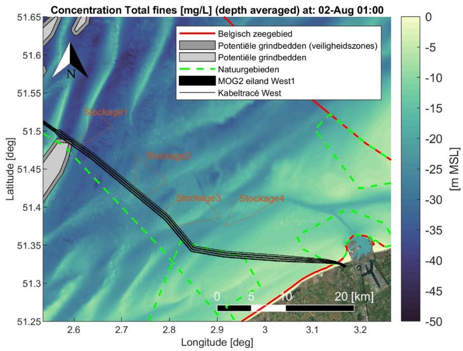
Figure Annex B-3 Map showing encountered depth averaged sediment concentration [mg/L] of fine material (< 250  $\mu\text{m}$ ) during a time instant of the simulation period. Scenario: Dredging cable trenches (trench1 section) and disposal at a temporary disposal site (Stockage3).
