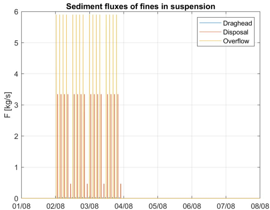
Figure Annex A-7 Timeseries of the implemented source of fines ( $d_p < 63 \mu\text{m}$ ) [kg/s] as a result dredging trenches at trench section 1 for the power cables and disposing dredged material at a temporary disposal site 3.
