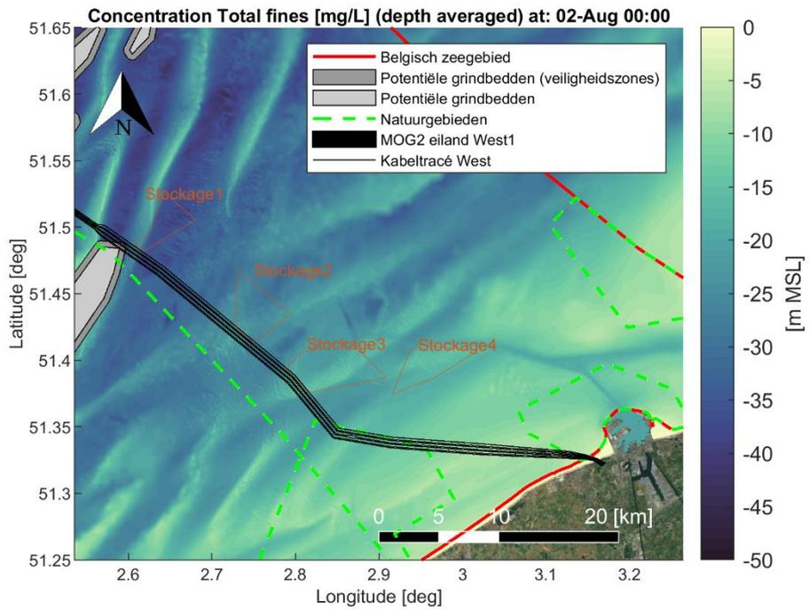
Figure Annex B-1 Map showing encountered depth averaged sediment concentration [mg/L] of fine material (< 250 [µm]) during a time instant of the simulation period. Scenario: Dredging cable trenches (trench1 section) and disposal at a temporary disposal site (Stockage3).
