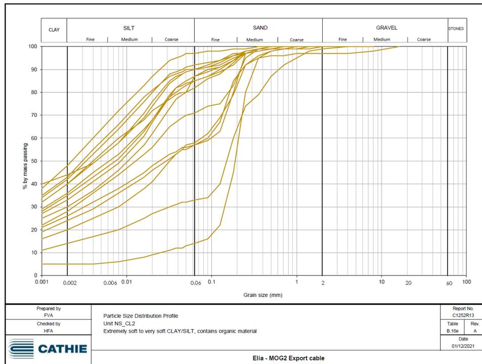
Figure 2-12 Particle size distribution profile of unit NS\_CL2 (extremely soft to very soft clay/silt, contains organic material), adapted from Cathie draft report (2021)
