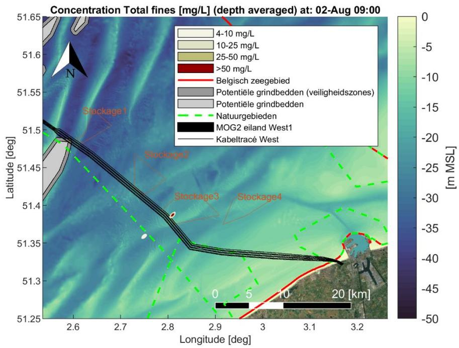
Figure Annex B-19 Map showing encountered depth averaged sediment concentration [mg/L] of fine material (< 250 [μm]) during a time instant of the simulation period. Scenario: Dredging cable trenches (trench1 section) and disposal at a temporary disposal site (Stockage3).
