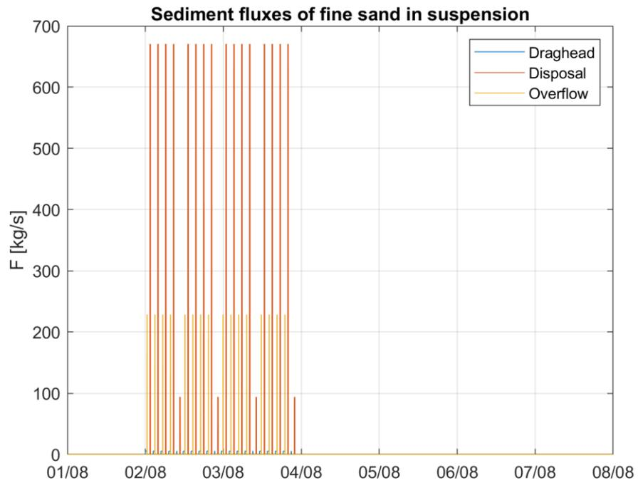
Figure Annex A-8 Timeseries of the implemented source of fine sand [kg/s] as a result dredging trenches at trench section 1 for the power cables and disposing dredged material at a temporary disposal site 3.
