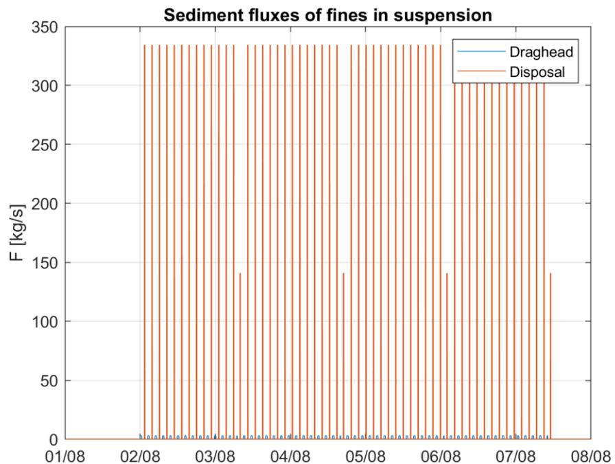
Figure Annex A-11 Time series of the implemented source of fines ( $d_p < 63 \mu\text{m}$ ) [ $\text{kg/s}$ ] as a result dredging trenches at trench section 3 for the power cables and disposing dredged material at a temporary disposal site 3.
