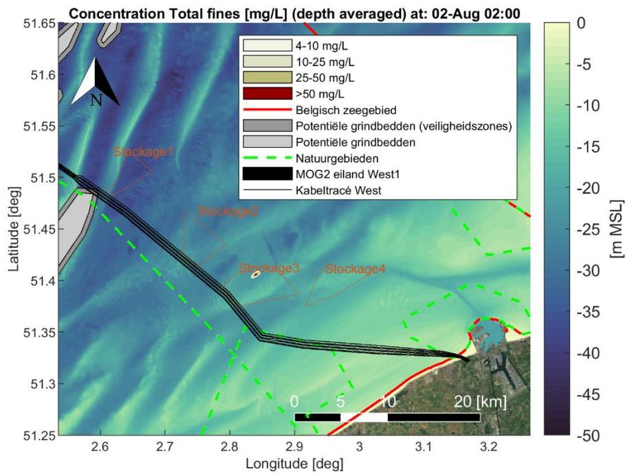
Figure Annex B-5 Map showing encountered depth averaged sediment concentration [mg/L] of fine material (< 250 [µm]) during a time instant of the simulation period. Scenario: Dredging cable trenches (trench1 section) and disposal at a temporary disposal site (Stockage3).
