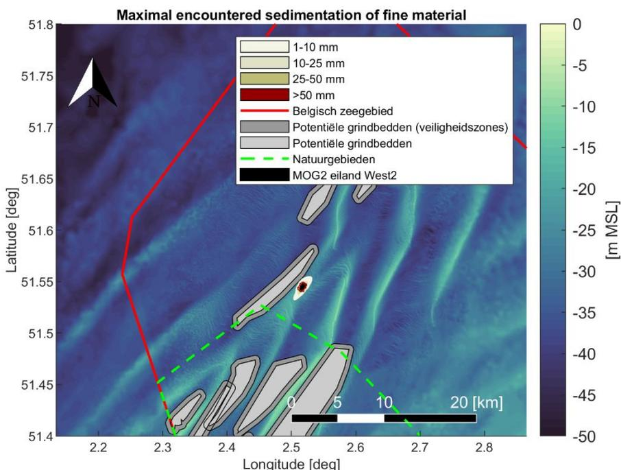
Figure 4-4 Maximal encountered sedimentation [mm] of fine material (< 250  $\mu\text{m}$ ) during the simulation period. Scenario 2: pre-dredging scour holes and creation of sand plateau at the island location West2.
