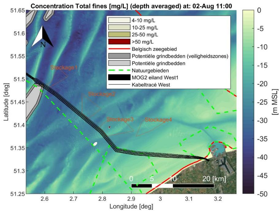
Figure Annex B-23 Map showing encountered depth averaged sediment concentration [mg/L] of fine material (< 250  $\mu\text{m}$ ) during a time instant of the simulation period. Scenario: Dredging cable trenches (trench1 section) and disposal at a temporary disposal site (Stockage3).
