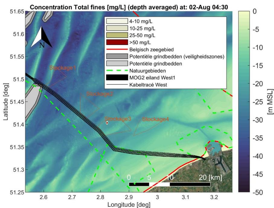
Figure Annex B-10 Map showing encountered depth averaged sediment concentration [mg/L] of fine material (< 250 [μm]) during a time instant of the simulation period. Scenario: Dredging cable trenches (trench1 section) and disposal at a temporary disposal site (Stockage3).
