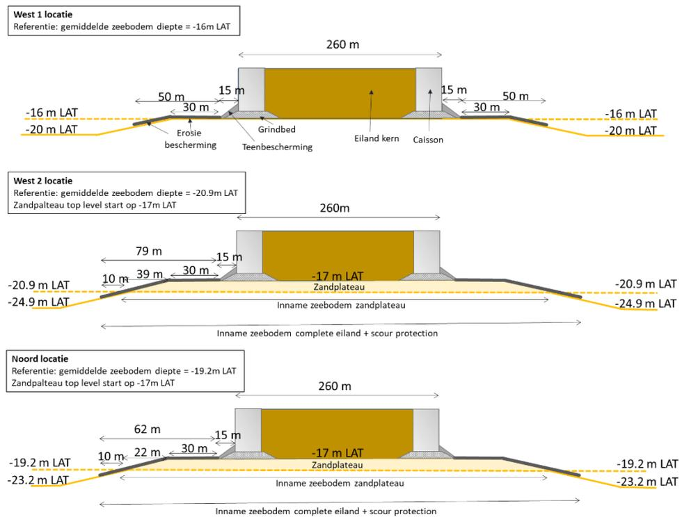
Figure 2-4 Cross-section of proposed island and scour protection dimensions for the West 1 (top), West 2 (mid) and Noord (bottom) location.
