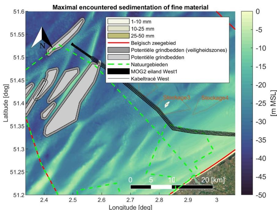
Figure 4-14 Maximal sedimentation [mm] of fine material (< 250  $\mu\text{m}$ ) during the simulation period. Scenario: Dredging cable trenches (trench1 section) and disposal at a temporary disposal site (Stockage3).
