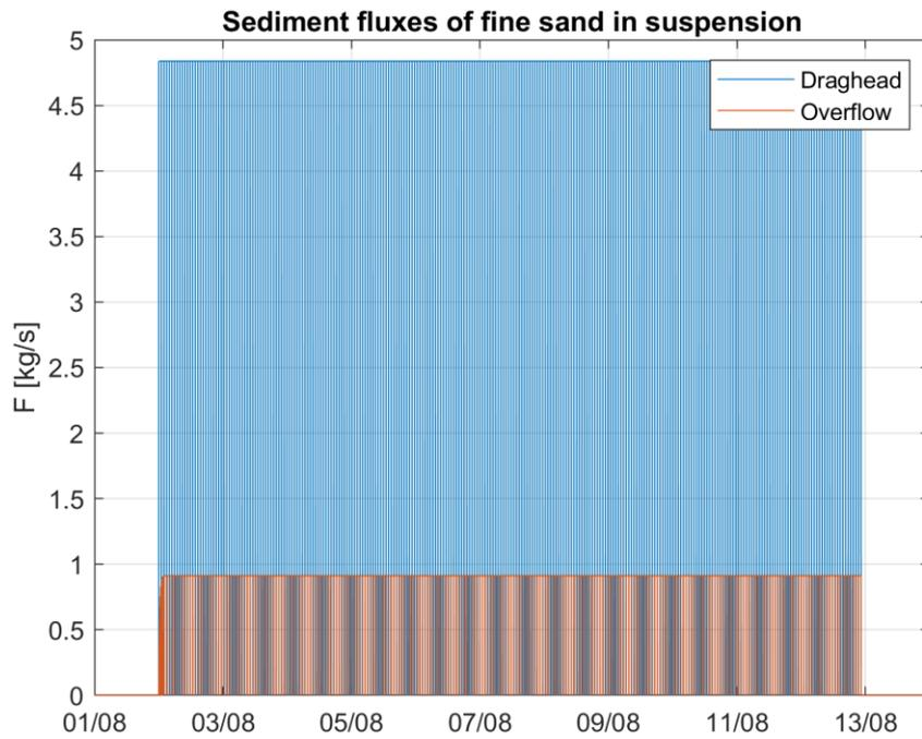
Figure Annex A-2 Time series of the implemented source of fine sand [ $\text{kg/s}$ ] as a result of pre-dredging scour holes and ridges and filling the island ring with dredged sand through pipes, leading to overflow from the island ring at the West 1 location.
