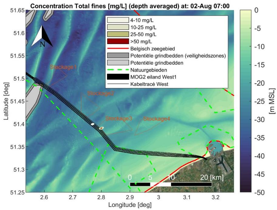
Figure Annex B-15 Map showing encountered depth averaged sediment concentration [mg/L] of fine material (< 250 [μm]) during a time instant of the simulation period. Scenario: Dredging cable trenches (trench1 section) and disposal at a temporary disposal site (Stockage3).
