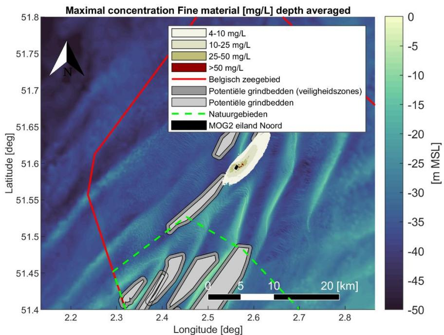
Figure 4-30 Maximal encountered depth averaged sediment concentration [mg/L] of fine material (< 250 [μm]) during the simulation period. Scenario: Plume generation and deposition as a result of natural erosion in one year time after Noord island construction, after one year case.
