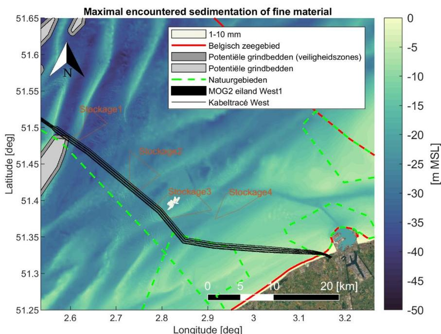
Figure 4-16 Maximal sedimentation [mm] of fine material (< 250  $\mu\text{m}$ ) during the simulation period. Scenario: Dredging cable trenches (trench 2 section) and disposal at a temporary disposal site (Stockage3).
