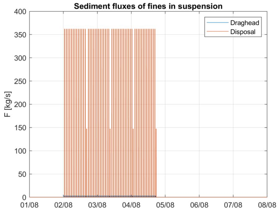
Figure Annex A-9 Timeseries of the implemented source of fines ( $d_p < 63 \mu\text{m}$ ) [kg/s] as a result dredging trenches at trench section 2 for the power cables and disposing dredged material at a temporary disposal site 3.
