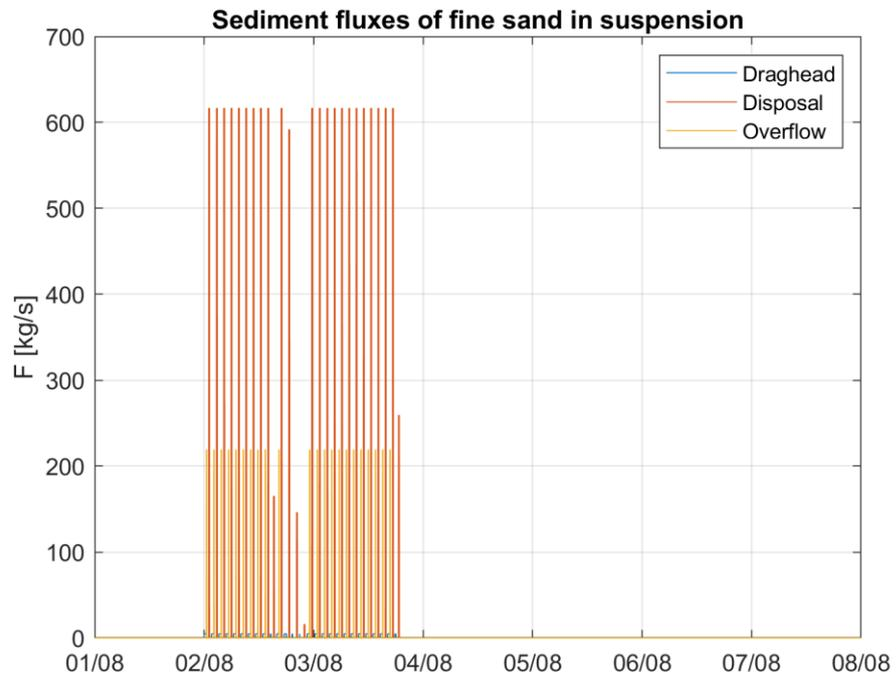
Figure 7-2 Time series of the implemented source of fine sand [kg/s] as a result of dredging works related to the levelling of sand ridge crests at the West 1 location.
