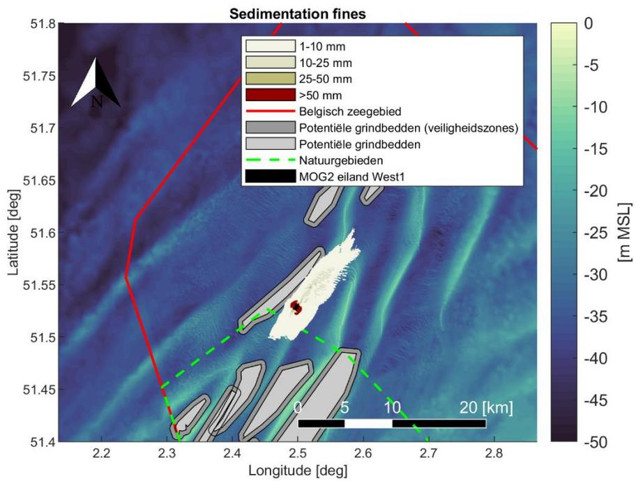
Figure 4-23 Maximal sedimentation [mm] of fine material (< 250 [μm]) during the simulation period. Scenario: : Plume generation and deposition as a result of natural erosion in one year time after West 1 island construction, after four year case.
