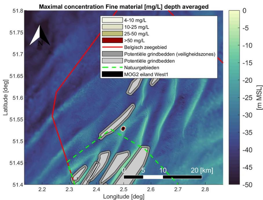
Figure 4-7 Maximal encountered depth averaged sediment concentration [mg/L] of fine material ( $< 250 [\mu m]$ ) during the simulation period. Scenario 3: pre-dredging scour holes and filling the West 1 island ring.
