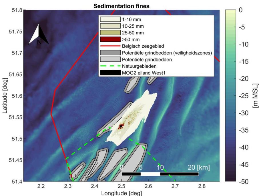
Figure 4-33 Maximal encountered sedimentation [mm] of fine material (< 250 µm) during the simulation period. Scenario: Plume generation and deposition as a result of natural erosion in one year time after West 1 island construction, after one year case including pre-scour design.
