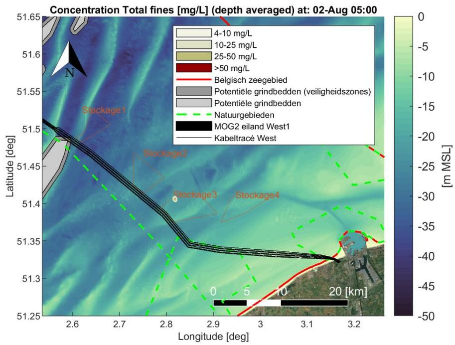
Figure Annex B-11 Map showing encountered depth averaged sediment concentration [mg/L] of fine material (< 250 [µm]) during a time instant of the simulation period. Scenario: Dredging cable trenches (trench1 section) and disposal at a temporary disposal site (Stockage3).
