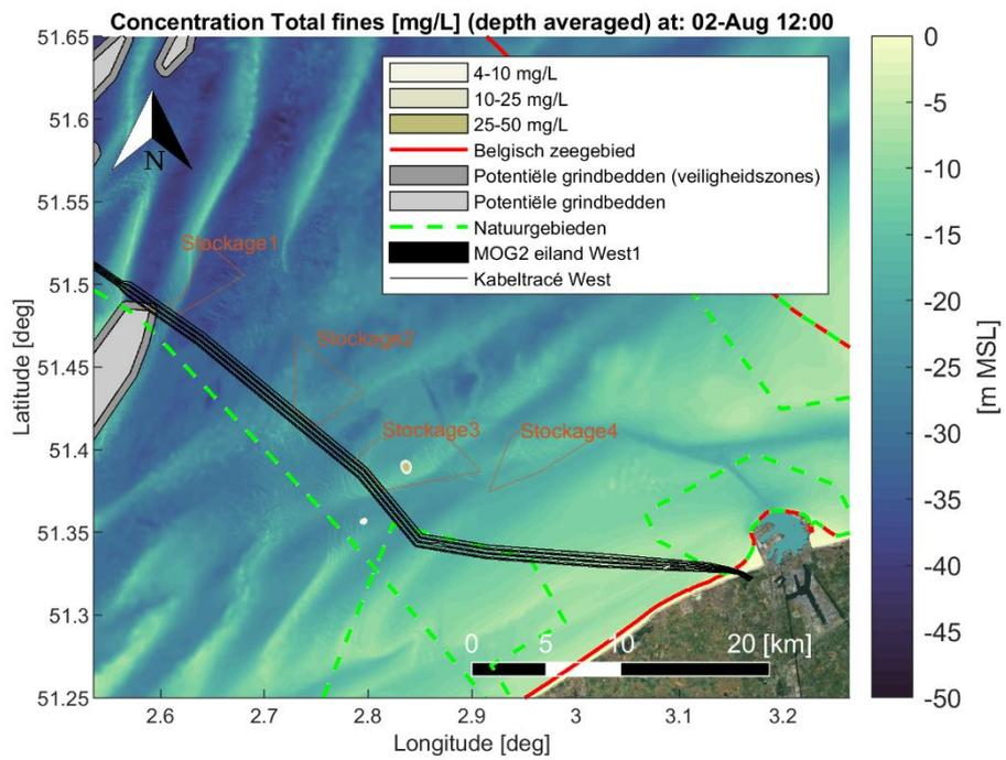
Figure Annex B-25 Map showing encountered depth averaged sediment concentration [mg/L] of fine material (< 250  $\mu\text{m}$ ) during a time instant of the simulation period. Scenario: Dredging cable trenches (trench1 section) and disposal at a temporary disposal site (Stockage3).
