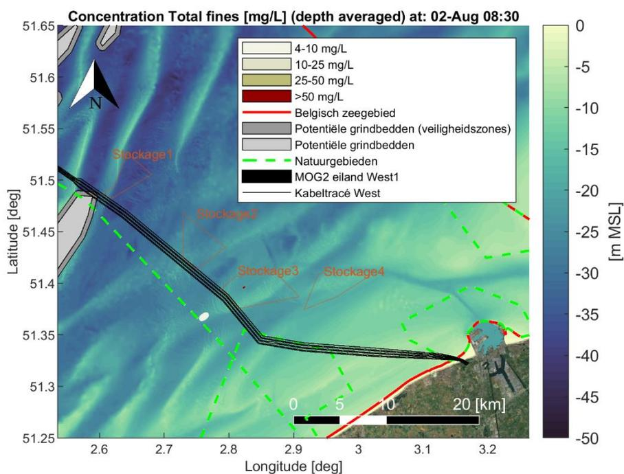
Figure Annex B-18 Map showing encountered depth averaged sediment concentration [mg/L] of fine material (< 250  $\mu\text{m}$ ) during a time instant of the simulation period. Scenario: Dredging cable trenches (trench1 section) and disposal at a temporary disposal site (Stockage3).
