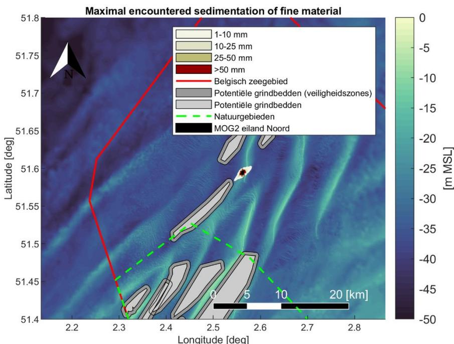
Figure 4-6 Maximal encountered sedimentation [mm] of fine material (< 250 [μm]) during the simulation period. Scenario 2: pre-dredging scour holes and creation of sand plateau at the island location Noord.
