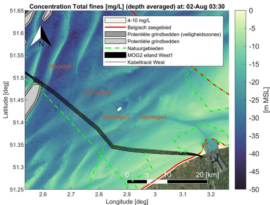
Figure Annex B-8 Map showing encountered depth averaged sediment concentration [mg/L] of fine material (< 250 [µm]) during a time instant of the simulation period. Scenario: Dredging cable trenches (trench1 section) and disposal at a temporary disposal site (Stockage3).
