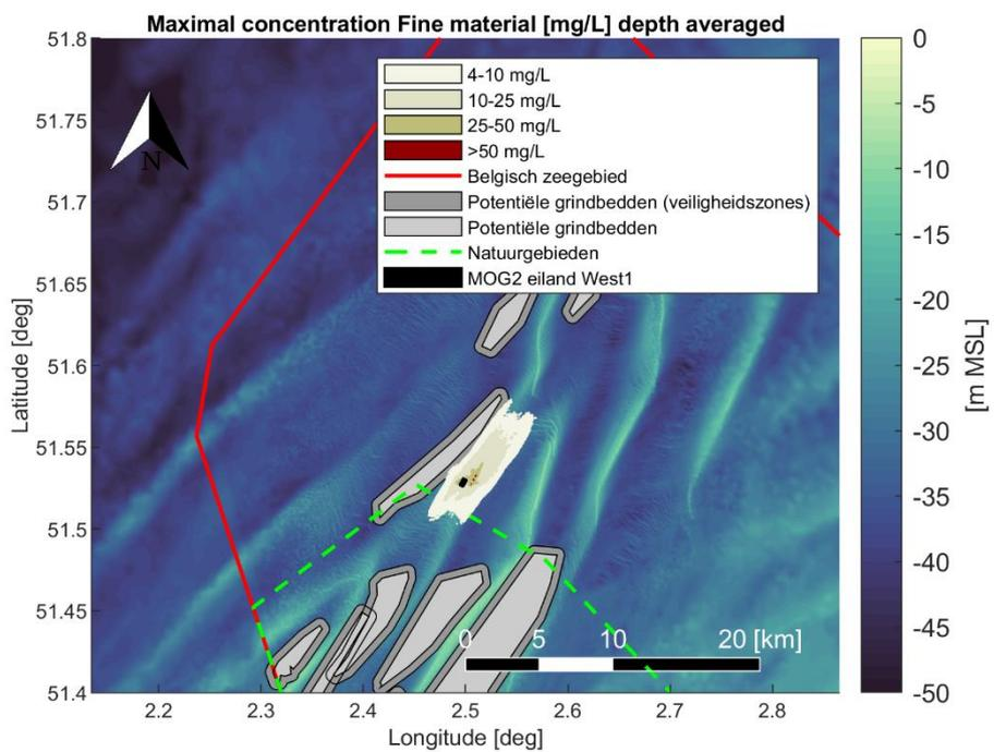
Figure 4-24 Maximal depth averaged sediment concentration [mg/L] of fine material (< 250 [μm]) during the simulation period. Scenario: : Plume generation and deposition as a result of natural erosion in one year time after West 1 island construction, after four year case..
