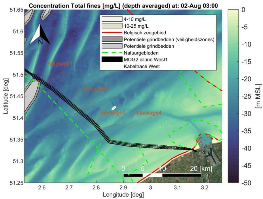
Figure Annex B-7 Map showing encountered depth averaged sediment concentration [mg/L] of fine material (< 250 [μm]) during a time instant of the simulation period. Scenario: Dredging cable trenches (trench1 section) and disposal at a temporary disposal site (Stockage3).
