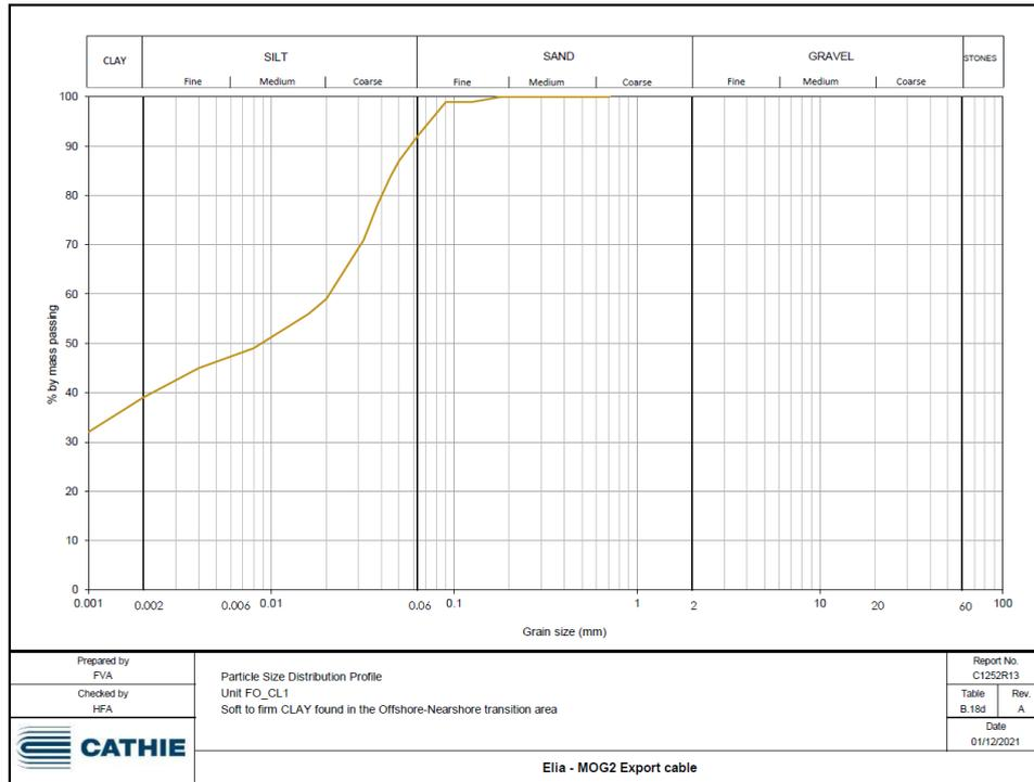
Figure 2-11 Particle size distribution profile of unit FO\_CL1 (soft to firm clay found in the offshore-nearshore transition zone), adapted from Cathie draft report (2021).
