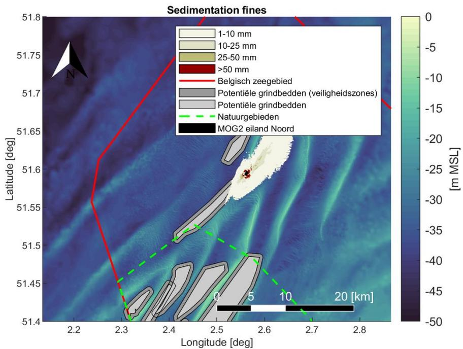
Figure 4-29 Maximal encountered sedimentation [mm] of fine material (< 250 [μm]) during the simulation period. Scenario: Plume generation and deposition as a result of natural erosion in one year time after Noord island construction, after one year case.
