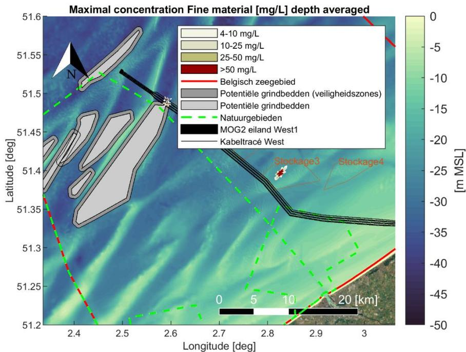
Figure 4-13 Maximal depth averaged sediment concentration [mg/L] of fine material (< 250 µm) during the simulation period. Scenario: Dredging cable trenches (trench1 section) and disposal at a temporary disposal site (Stockage3).
