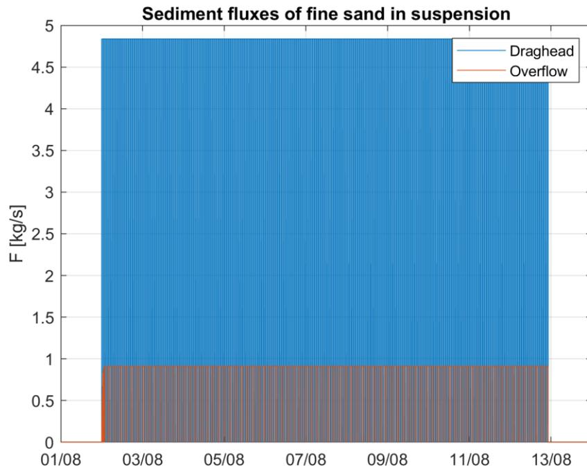
Figure Annex A-4 Time series of the implemented source of fine sand [ $\text{kg/s}$ ] as a result of pre-dredging scour holes and ridges and filling the island ring with dredged sand through pipes, leading to overflow from the island ring at the West 2 location.
