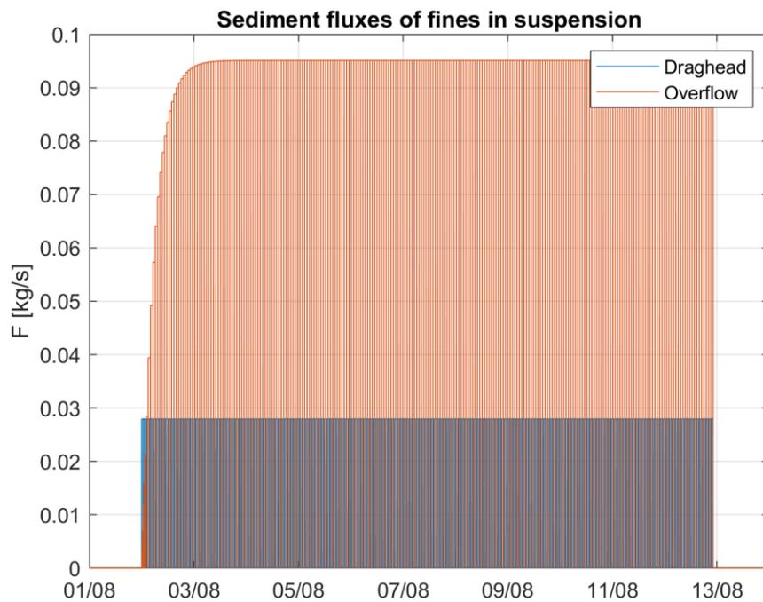
Figure Annex A-5 Time series of the implemented source of fines ( $d_p < 63 \mu\text{m}$ ) [ $\text{kg/s}$ ] as a result of pre-dredging scour holes and ridges and filling the island ring with dredged sand through pipes, leading to overflow from the island ring at the Noord location.
