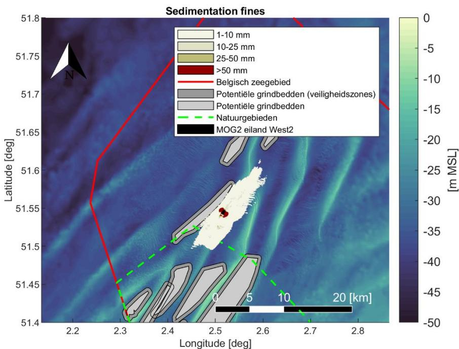
Figure 4-27 Maximal encountered sedimentation [mm] of fine material (< 250 [μm]) during the simulation period. Scenario: Plume generation and deposition as a result of natural erosion in one year time after West 2 island construction, after four year case.
