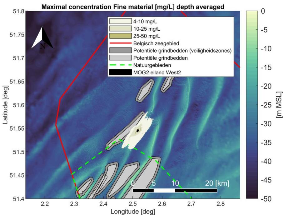
Figure 4-26 Maximal encountered depth averaged sediment concentration [mg/L] of fine material (< 250 [μm]) during the simulation period. Scenario: Plume generation and deposition as a result of natural erosion in one year time after West 2 island construction, after one year case.
