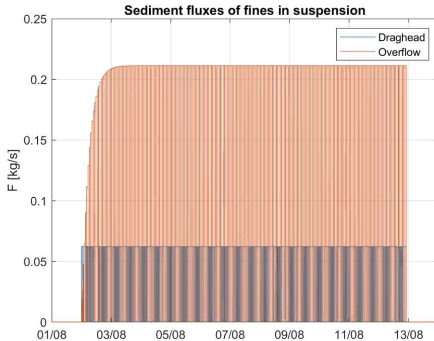
Figure Annex A-1 Time series of the implemented source of fines ( $d_p < 63 \mu\text{m}$ ) [kg/s] as a result of pre-dredging scour holes and ridges and filling the island ring with dredged sand through pipes, leading to overflow from the island ring at the West 1 location.
