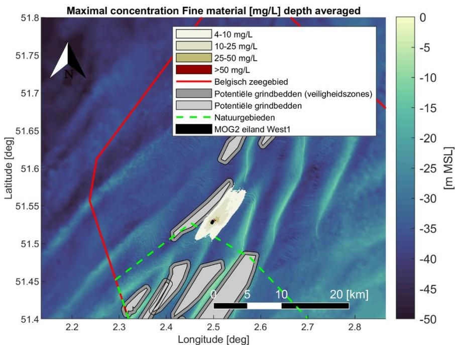
Figure 4-22 Maximal depth averaged sediment concentration [mg/L] of fine material (< 250 [μm]) during the simulation period. Scenario: : Plume generation and deposition as a result of natural erosion in one year time after West 1 island construction, after one year case..
