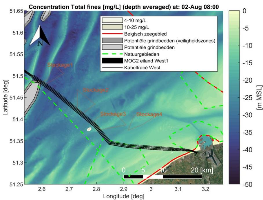
Figure Annex B-17 Map showing encountered depth averaged sediment concentration [mg/L] of fine material (< 250 [μm]) during a time instant of the simulation period. Scenario: Dredging cable trenches (trench1 section) and disposal at a temporary disposal site (Stockage3).
