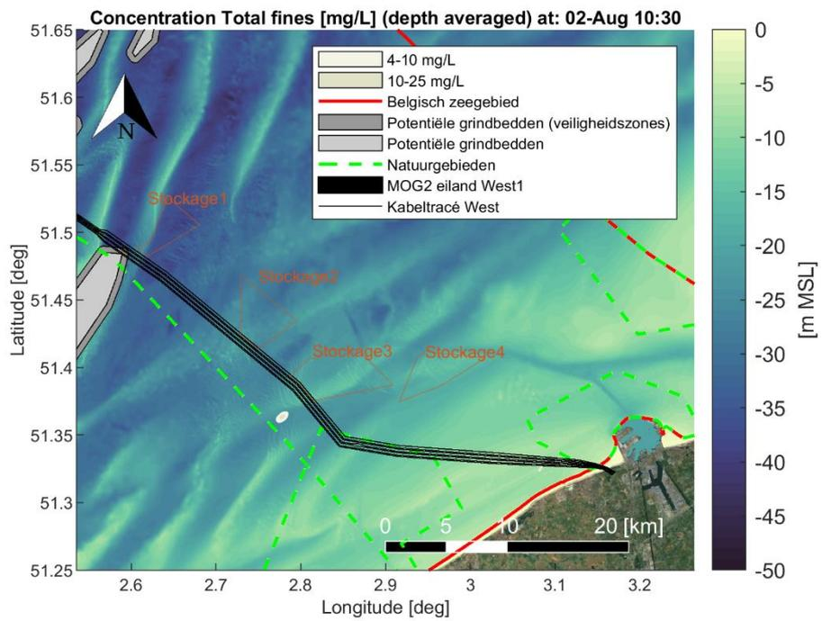
Figure Annex B-22 Map showing encountered depth averaged sediment concentration [mg/L] of fine material (< 250 [μm]) during a time instant of the simulation period. Scenario: Dredging cable trenches (trench1 section) and disposal at a temporary disposal site (Stockage3).
