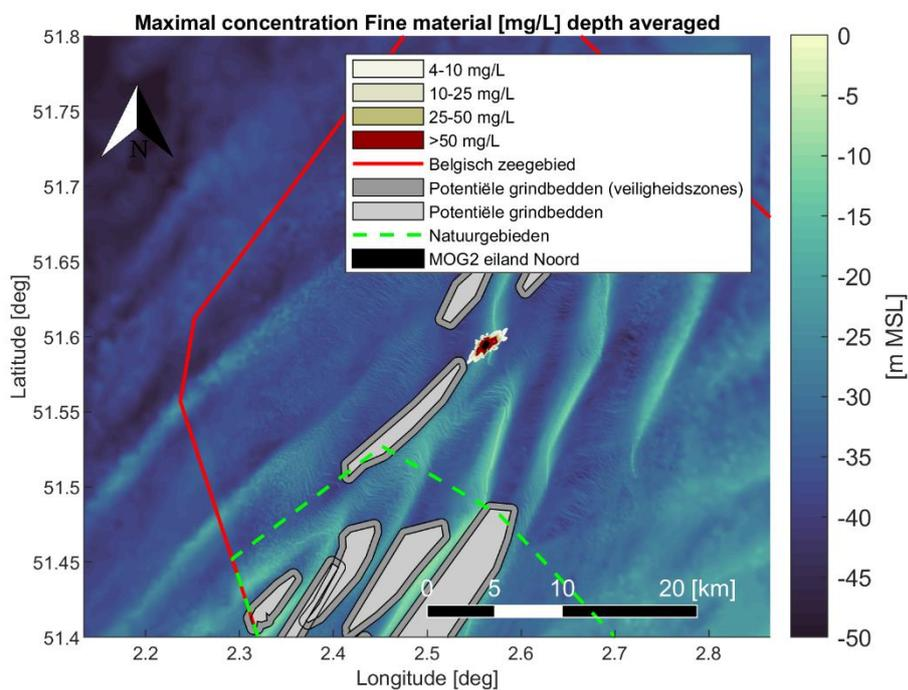
Figure 4-5 Maximal encountered depth averaged sediment concentration [mg/L] of fine material ( $< 250 [\mu m]$ ) during the simulation period. Scenario 2: pre-dredging scour holes and creation of sand plateau at the island location Noord.
