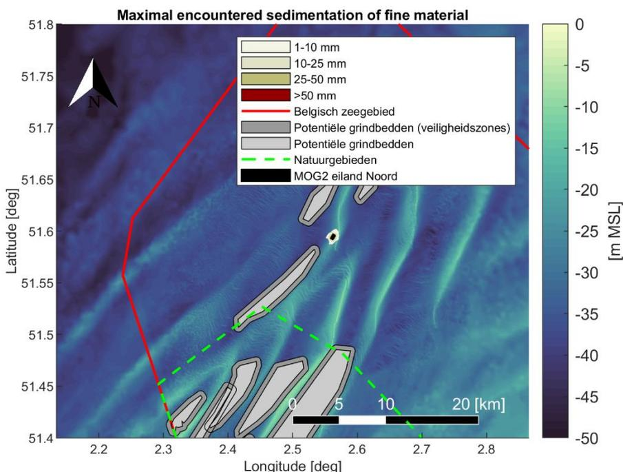
Figure 4-12 Maximal encountered sedimentation [mm] of fine material (< 250 [µm]) during the simulation period. Scenario 3: pre-dredging scour holes and filling the Noord island ring.
