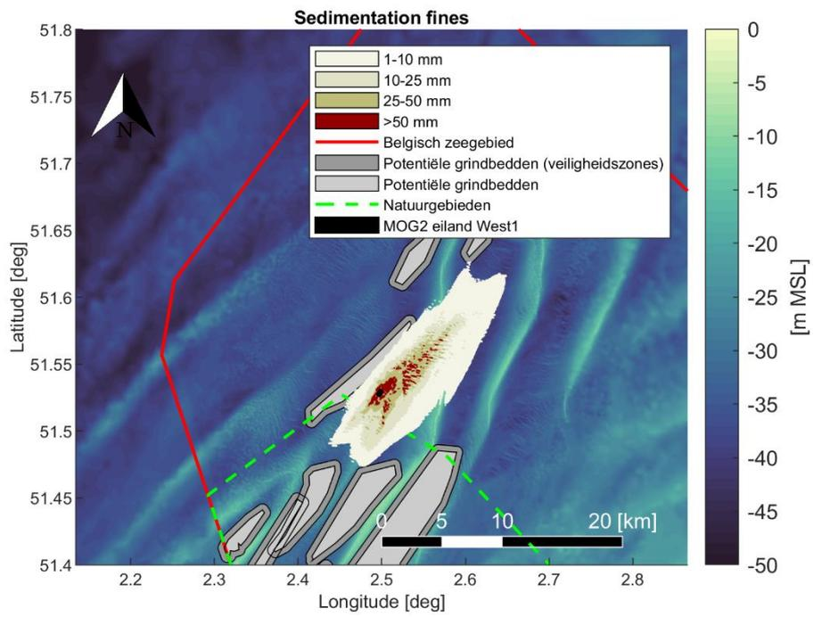
Figure 4-34 Maximal encountered sedimentation [mm] of fine material (< 250 [μm]) during the simulation period. Scenario: Plume generation and deposition as a result of natural erosion in one year time after West 1 island construction, after one year case without pre-scour design.
