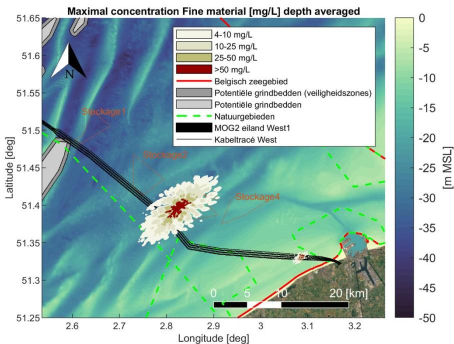
Figure 4-17 Maximal encountered depth averaged sediment concentration [mg/L] of fine material (< 250 µm) during the simulation period. Scenario: Dredging cable trenches (trench 3 section) and disposal at a temporary disposal site (Stockage3).
