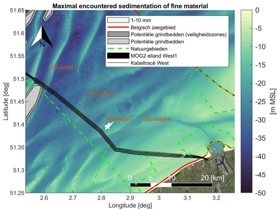
Figure 4-18 Maximal sedimentation [mm] of fine material (< 250 [μm]) during the simulation period. Scenario: Dredging cable trenches (trench 3 section) and disposal at a temporary disposal site (Stockage3).
