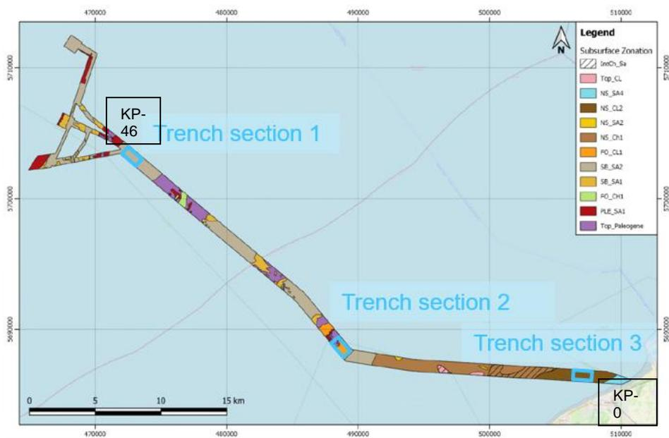
Figure 3-2 Subsurface sediment unitization, adapted from Cathie draft report (2021) along the power cable track and locations of simulated trench sections.
