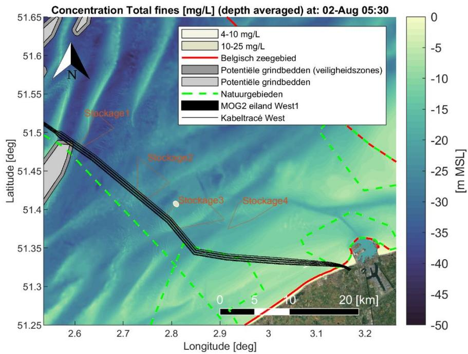
Figure Annex B-12 Map showing encountered depth averaged sediment concentration [mg/L] of fine material (< 250 [μm]) during a time instant of the simulation period. Scenario: Dredging cable trenches (trench1 section) and disposal at a temporary disposal site (Stockage3).
