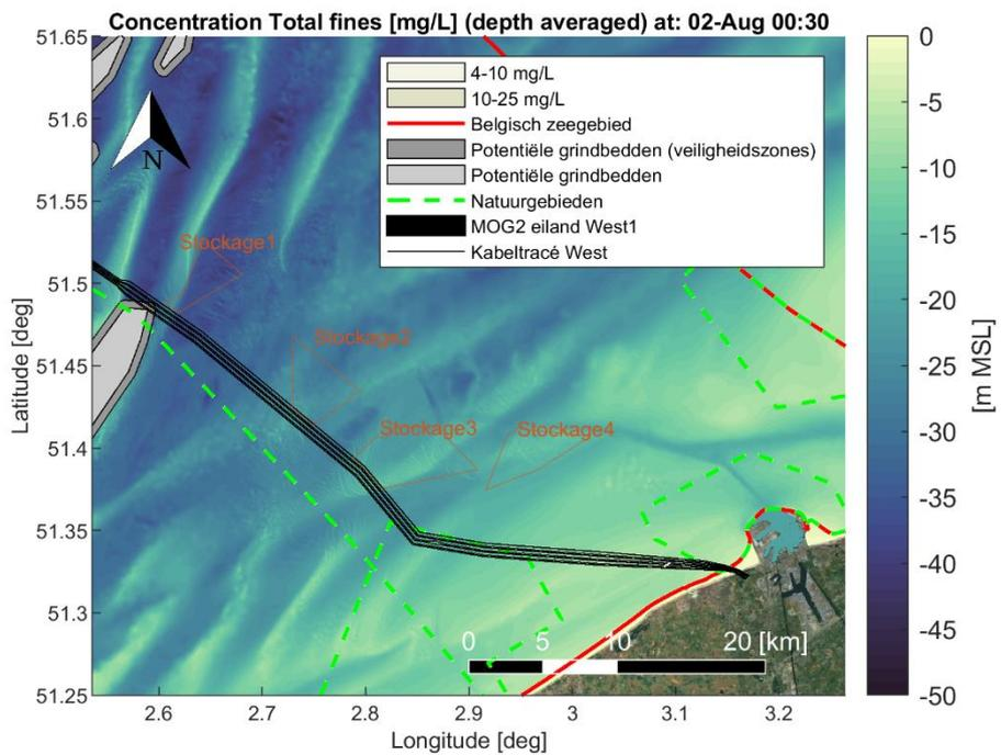
Figure Annex B-2 Map showing encountered depth averaged sediment concentration [mg/L] of fine material (< 250 [µm]) during a time instant of the simulation period. Scenario: Dredging cable trenches (trench1 section) and disposal at a temporary disposal site (Stockage3).
