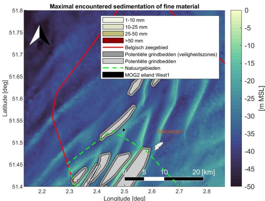
Figure 4-2 Maximal encountered sedimentation [mm] of fine material (< 250 [µm]) during the simulation period. Scenario 1: levelling sand ridges and disposal at a temporary disposal site (island location West 1).
