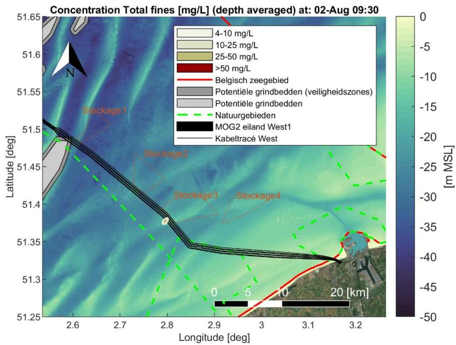
Figure Annex B-20 Map showing encountered depth averaged sediment concentration [mg/L] of fine material (< 250 [μm]) during a time instant of the simulation period. Scenario: Dredging cable trenches (trench1 section) and disposal at a temporary disposal site (Stockage3).
