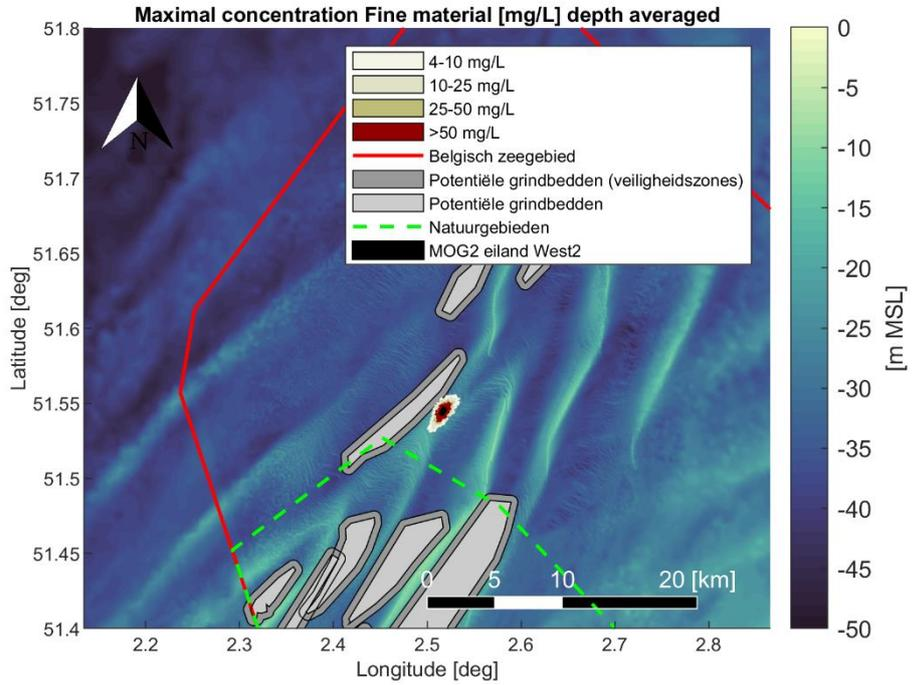
Figure 4-3 Maximal encountered depth averaged sediment concentration [mg/L] of fine material ( $< 250 \mu m$ ) during the simulation period. Scenario: Plume generation while pre-dredging scour holes and ridges and disposing dredged material at the island location West 2.
