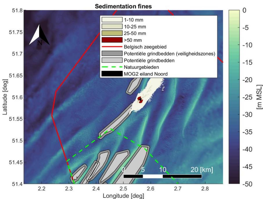
Figure 4-31 Maximal encountered sedimentation [mm] of fine material (< 250 [μm]) during the simulation period. Scenario: Plume generation and deposition as a result of natural erosion in one year time after Noord island construction, after four year case.
