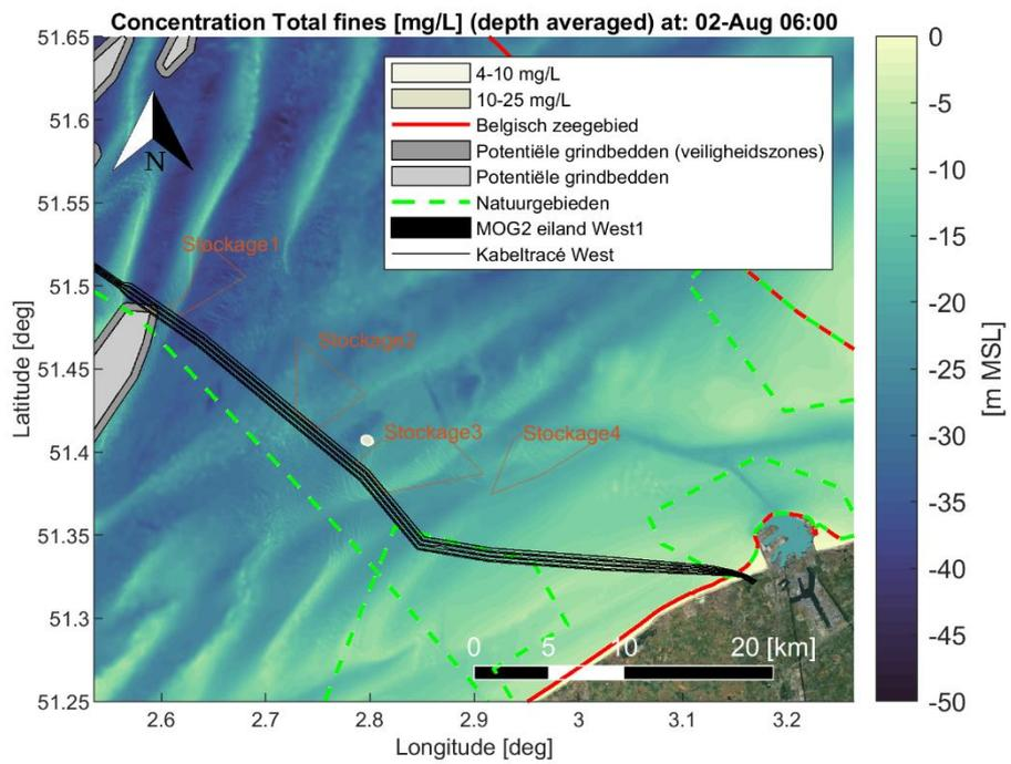
Figure Annex B-13 Map showing encountered depth averaged sediment concentration [mg/L] of fine material (< 250 [µm]) during a time instant of the simulation period. Scenario: Dredging cable trenches (trench1 section) and disposal at a temporary disposal site (Stockage3).
