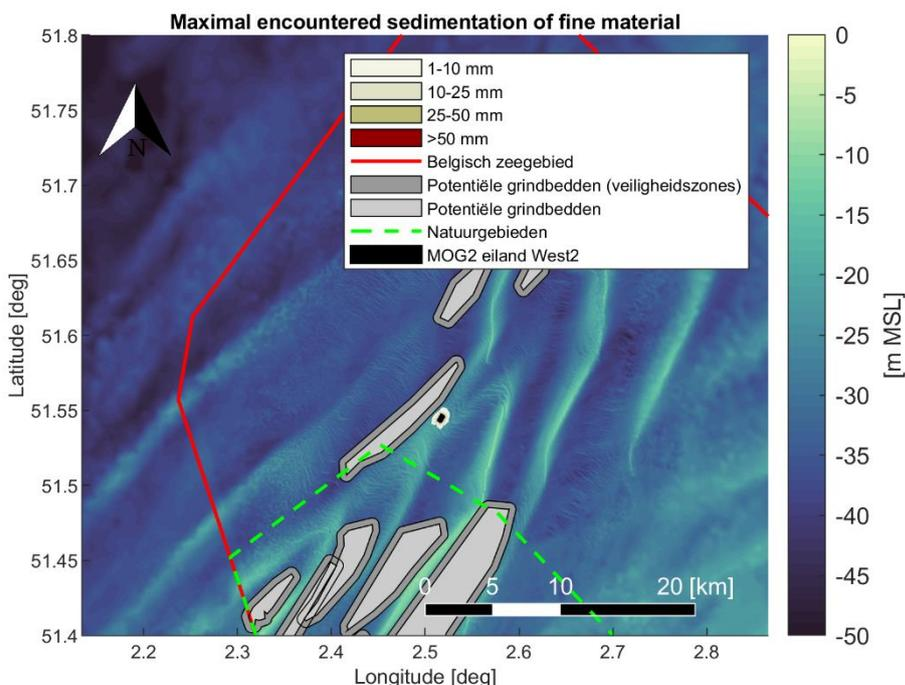
Figure 4-10 Maximal encountered sedimentation [mm] of fine material (< 250 [μm]) during the simulation period. Scenario 3: pre-dredging scour holes and filling the West 2 island ring.
