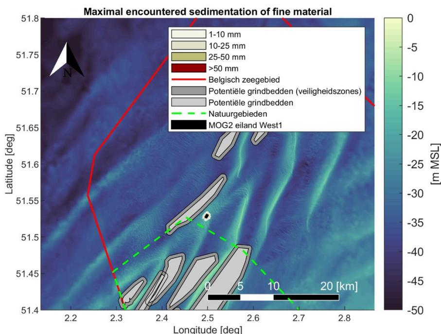
Figure 4-8 Maximal encountered sedimentation [mm] of fine material (< 250  $\mu\text{m}$ ) during the simulation period. Scenario 3: pre-dredging scour holes and filling the West 1 island ring.
