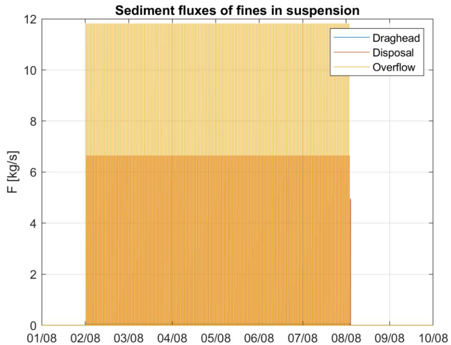
Figure 7-3 Time series of the implemented source of fines ( $d_p < 63 \mu\text{m}$ ) [kg/s] as a result of pre-dredging scour holes and ridges and disposing dredged material at the island location at the West 2 location.
