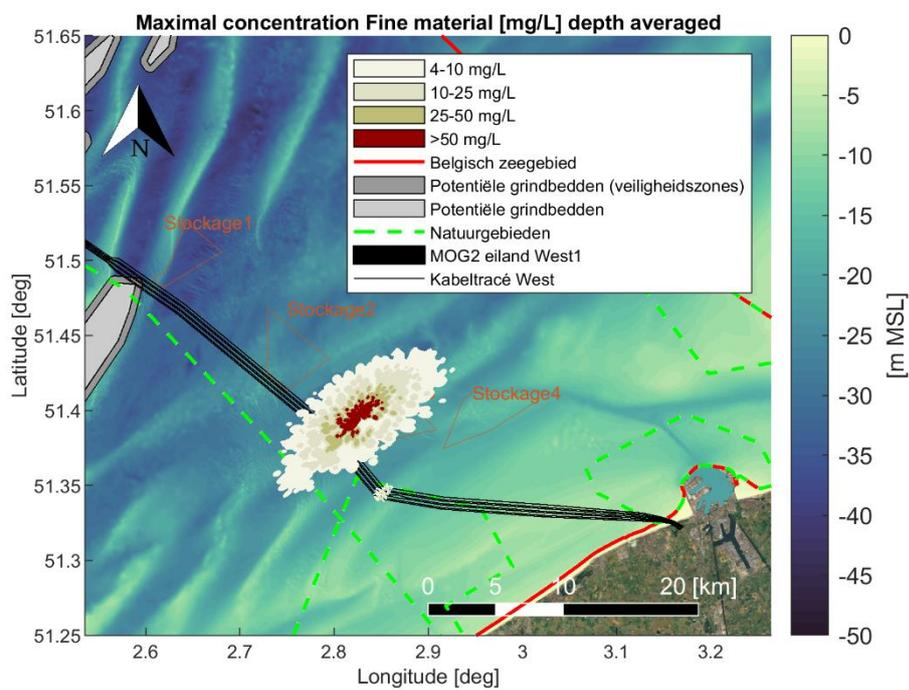
Figure 4-15 Maximal depth averaged sediment concentration [mg/L] of fine material (< 250 µm) during the simulation period. Scenario: Dredging cable trenches (trench 2 section) and disposal at a temporary disposal site (Stockage3).
