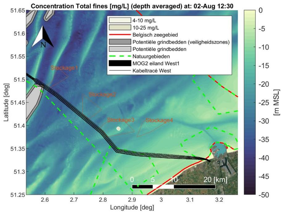
Figure Annex B-26 Map showing encountered depth averaged sediment concentration [mg/L] of fine material (< 250 [μm]) during a time instant of the simulation period. Scenario: Dredging cable trenches (trench1 section) and disposal at a temporary disposal site (Stockage3).
