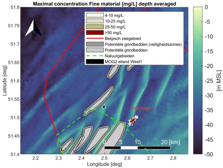
Figure 4-1 Maximal encountered depth averaged sediment concentration [mg/L] of fine material ( $< 250 [\mu m]$ ) during the simulation period Scenario 1: levelling sand ridges and disposal at a temporary disposal site (island location West 1).
