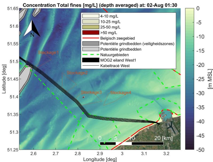
Figure Annex B-4 Map showing encountered depth averaged sediment concentration [mg/L] of fine material (< 250 [µm]) during a time instant of the simulation period. Scenario: Dredging cable trenches (trench1 section) and disposal at a temporary disposal site (Stockage3).
