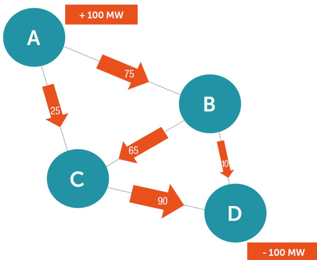
Figure 25 Example: Commercial exchanges between two countries can generate physical flows through other borders (resulting physical flows from an energy exchange of 100 MW between 2 zones).
