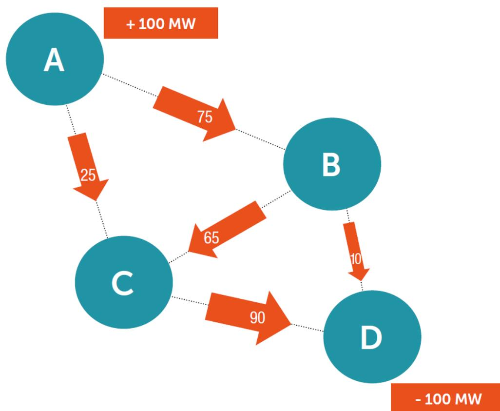
Figure 22 Example: Commercial exchanges between two countries can generate physical flows through other borders (resulting physical flows from an energy exchange of 100 MW between 2 zones).
