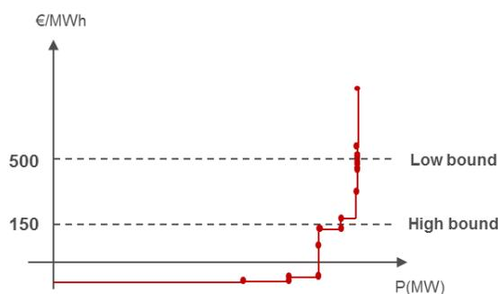
Figure 25: analysis of the supply aggregated curve
