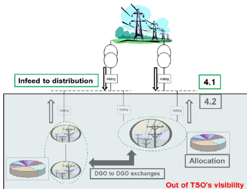
Figure 1: schematic view on the infeed metering
