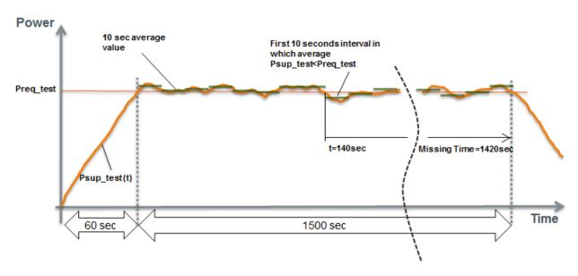
In the example hereabove, the ramping phase starts at t = 0 second. The interval during which the first  $AV_{FCR\ Power\ supplied}(10s\ window)$  inferior to the FCR Capacity Requested starts at t = 140 seconds. Taking into account that the energy availability test ends at t = 1560 seconds, the FCR Missing Time for the example amounts 1420 seconds.
