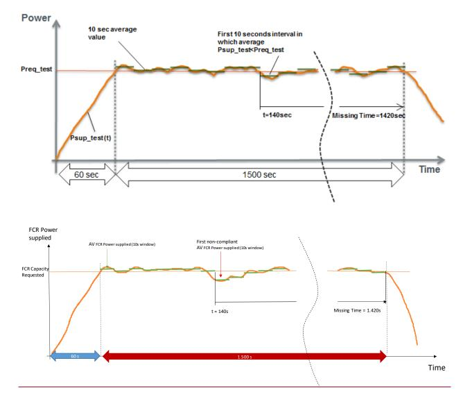
In the example hereabove, the ramping phase starts at t = 0 second. The interval during which the first  $AV_{FCR Power supplied}(10s window)$  is inferior to the FCR Capacity Requested starts at t = 140 seconds. Taking into account that the energy availability test ends at  $t = \frac{15601560}{560}$  seconds, the FCR Missing Time for the example amounts  $\frac{14201420}{500}$  seconds.
