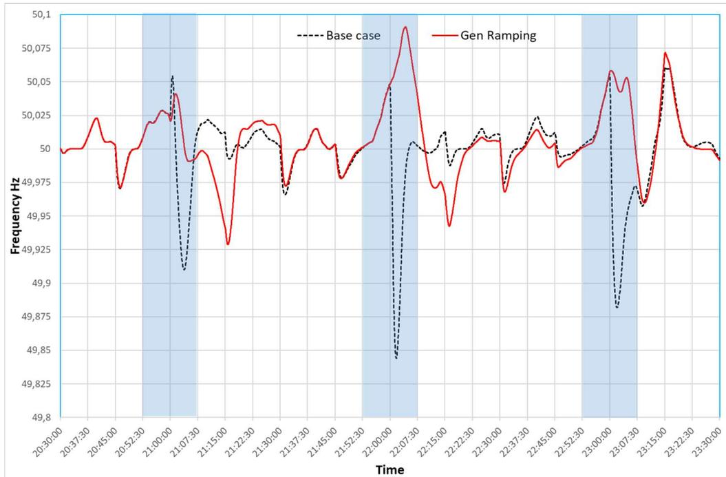
**Fig. 52 – Simulated frequency profile of the ramping on generation case compared to the reference base case scenario profile**
