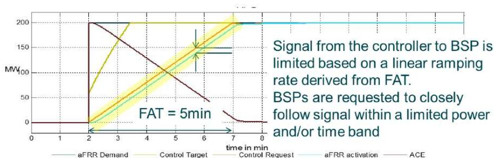
***Fig. 50 – aFRR activation method: ramping approach***
