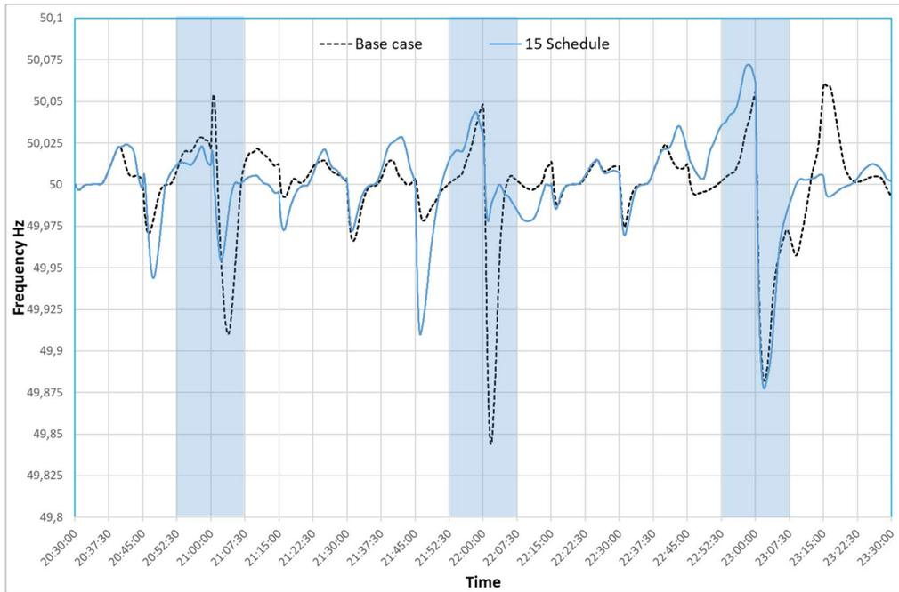
**Fig. 42 – Simulated frequency profile of the 15 min MTU compared to the reference base case scenario profile**
