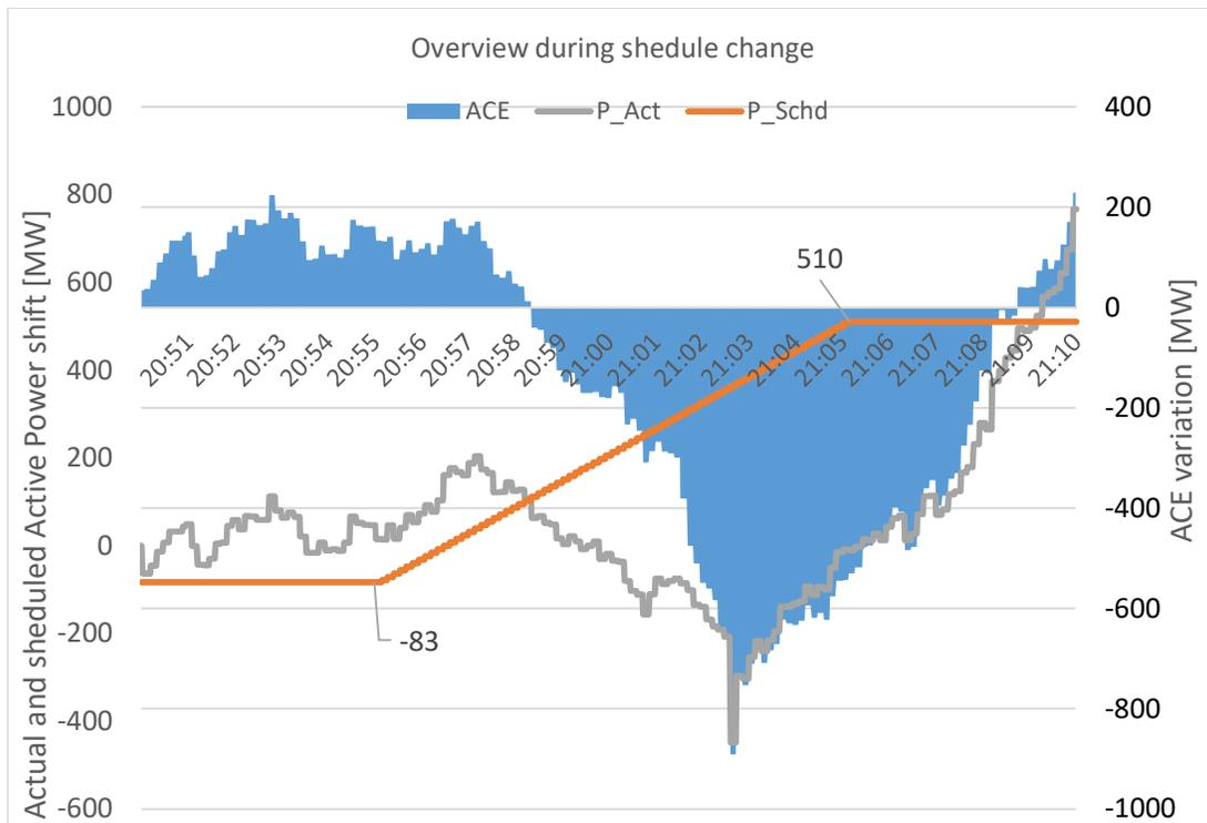
**Figure 17** Cross-border flow comparison between schedules and actual power exchange
