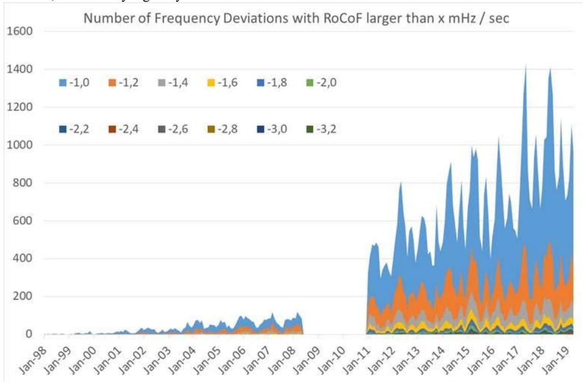
The higher levels of RoCoF above 2.2 mHz / sec are magnified in the graph below, as these are most relevant to observe the amplitude of the problem.
