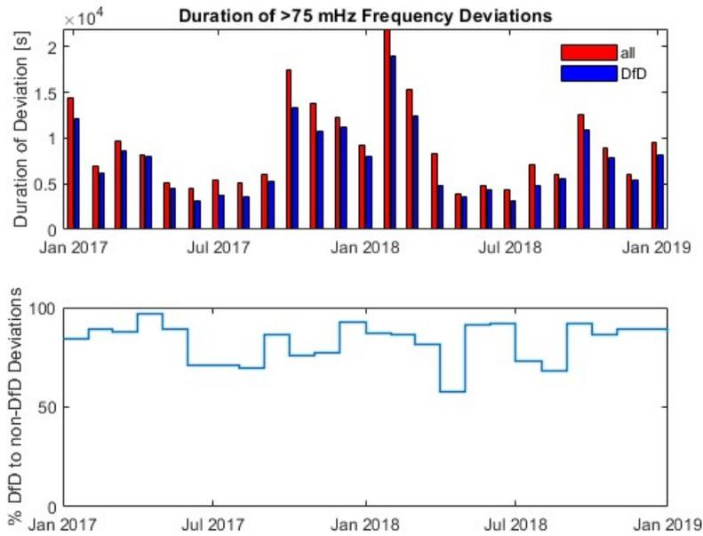
*Figure 4 – Duration of DFDs and % of DFD compared to all deviations in the last 2 years (>75 mHz)*
