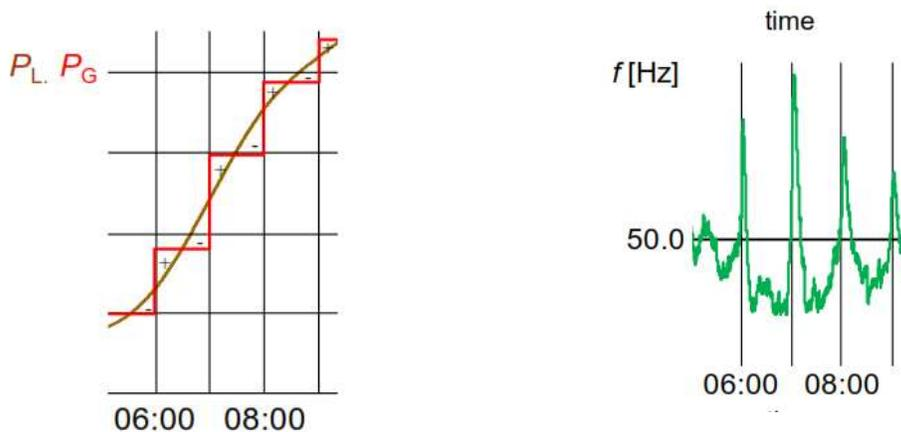
Figure 12– Effect of difference between load and schedules on frequency
