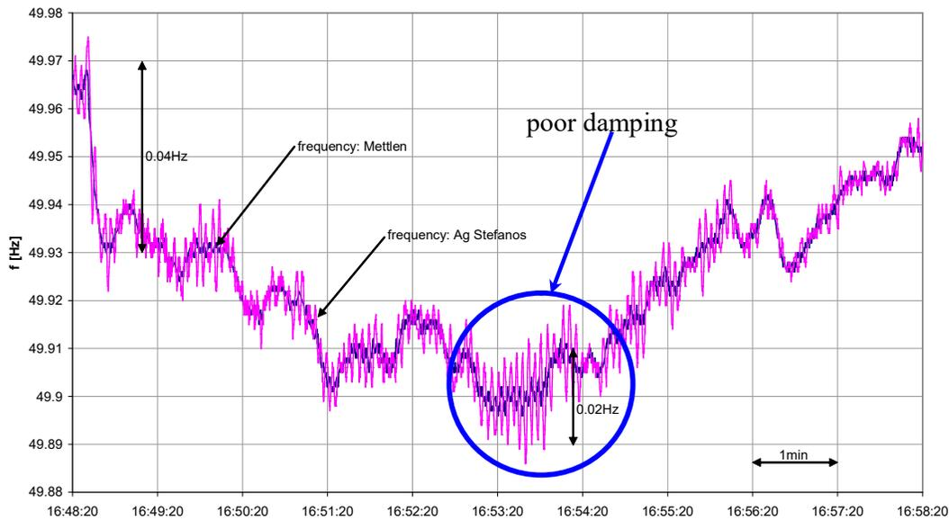
Figure 8 – Recording of poor damping of inter-area oscillations during frequency excursion [1]
