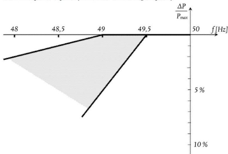
Figure 9 – Admissible power reduction under falling frequency [2]
