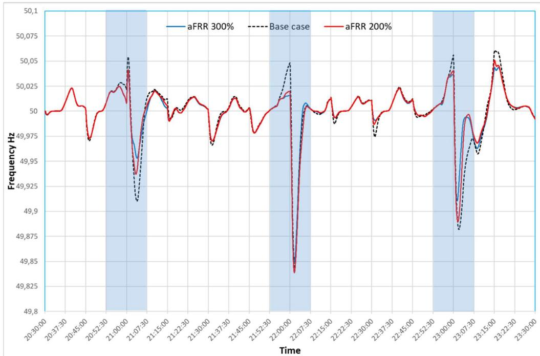
**Fig. 48 – Simulated frequency profile of the aFRR increase cases compared to the reference base case scenario profile**
