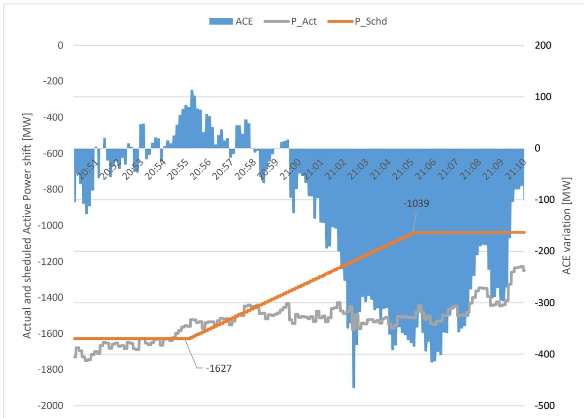
**Figure 30 Cross-border flow comparison between schedules and actual power exchange**
