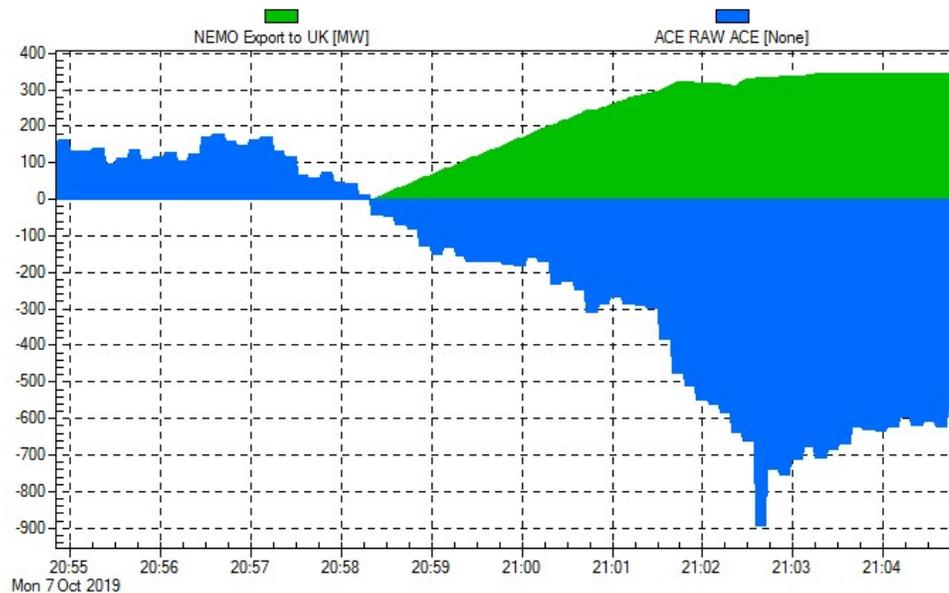
*Figure 20 Nemo measured active power ramping during the DfD*
