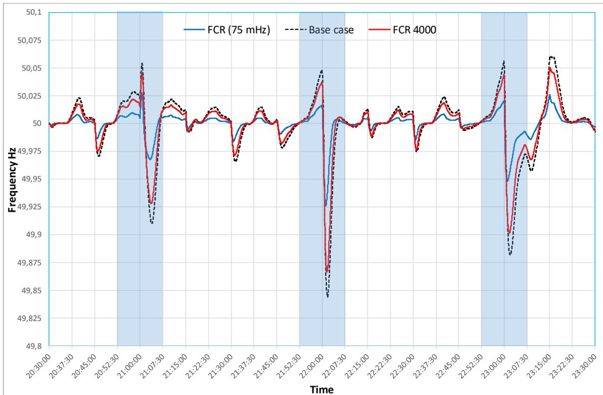
**Fig. 46 – Simulated frequency profile of the FCR increase cases compared to the reference base case scenario profile**
