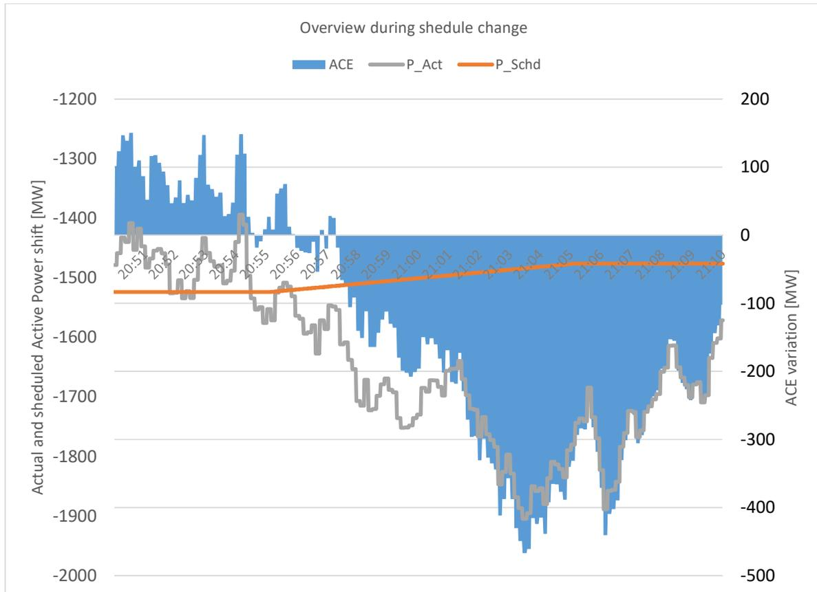
**Figure 23 Cross-border flow comparison between schedules and actual power exchange**
