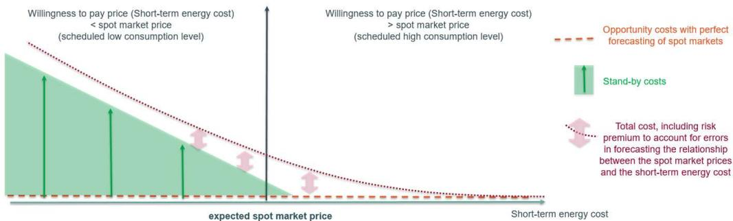
5c. Marginal cost of upward FRR capacity on consumption assets
