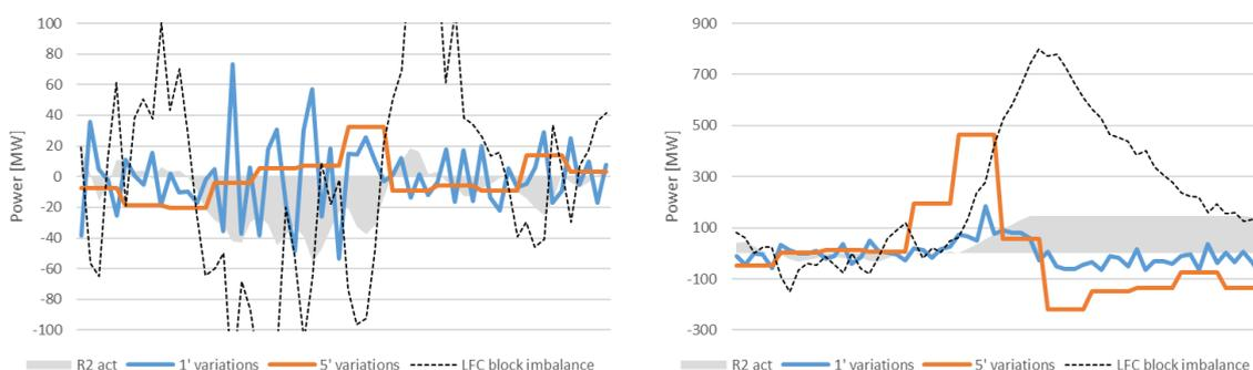
Figure 27: historic observations of aFRR activations (R2 act, positive values represent downward activations), and the LFC block imbalance, as well as the 1' and 5' variations of the remaining LFC block imbalances after IGCC activations (positive values represent excess energy) for a day with usual imbalances (May 17 2020) and high imbalances (May 14 2020).
