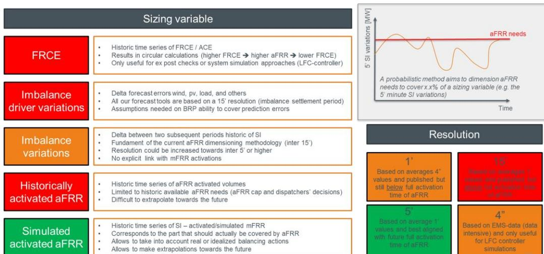
Figure 16: Overview of sizing variables and resolution options
