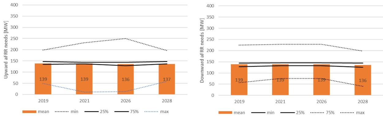
Figure 41: average, min / max and 25% - 75% percentile of the upward (left) and downward (right) aFRR needs towards 2028 for the reference case
