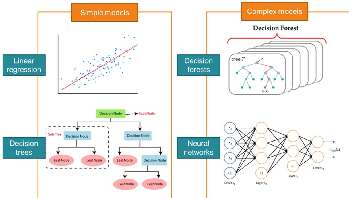
Figure 36: Graphical illustration of a linear regression (upper left), a decision tree (lower left), a random forest (upper right) and neural networks (down right).
