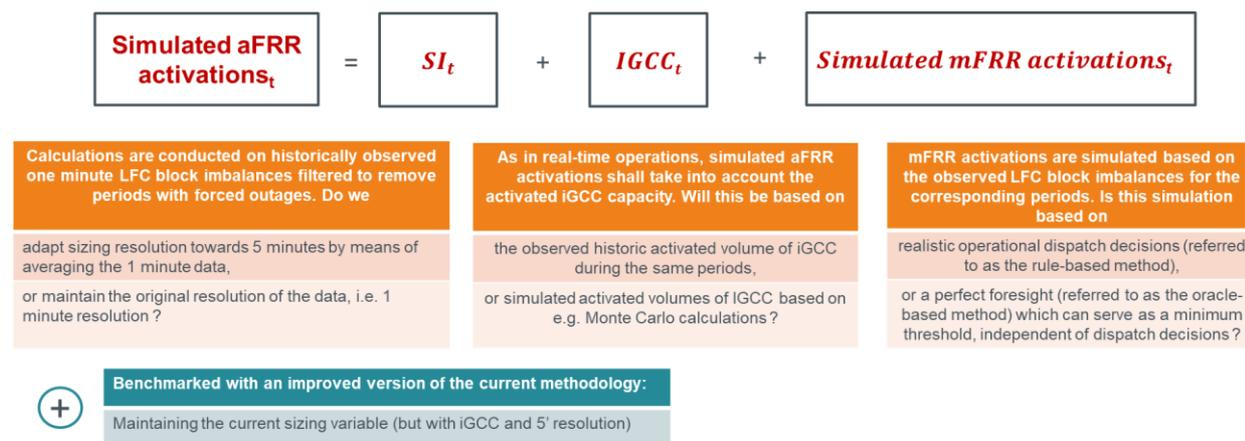
Figure 23: Calculation of the sizing variable “simulated aFRR activations” for every period t and analyzed methodology design options. Note that a positive (negative) LFC block imbalance (SI) refers to an excess (shortage) while a positive (negative) IGCC, simulated mFRR activation and aFRR activation refers to an upward (downward) activation
