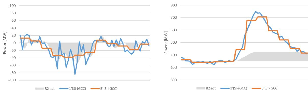
Figure 28: historic observations of aFRR activations (R2 act), and LFC block imbalances corrected with IGCC activations (SI-IGCC) with a resolution of 1' and 5' minutes for a day with usual imbalances (May 17 2020) and high imbalances (May 14 2020). Negative values represent a shortage or upward aFRR activation
