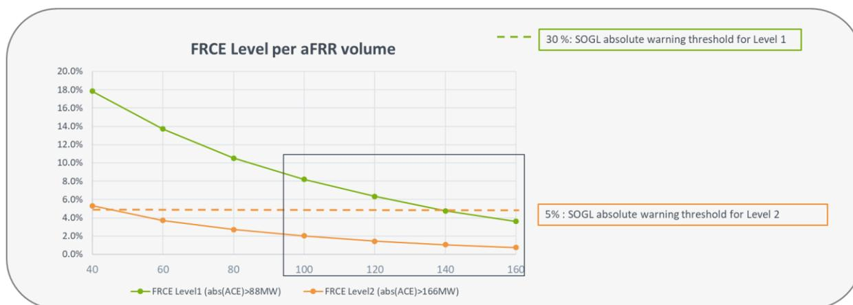
Figure 20: Impact of different aFRR availability on the Level 1 and Level 2 criteria
