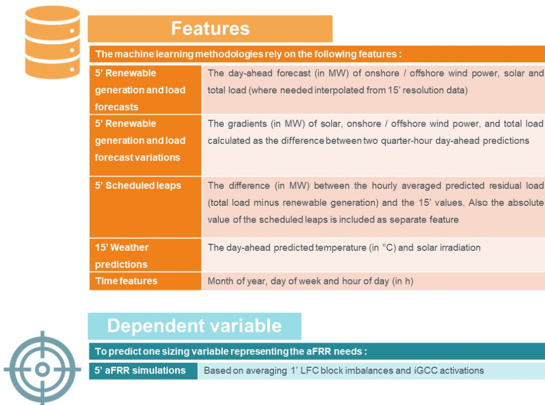
Figure 30: Overview of features (independent variables) and outcome (dependent variable) used by the machine learning algorithms
