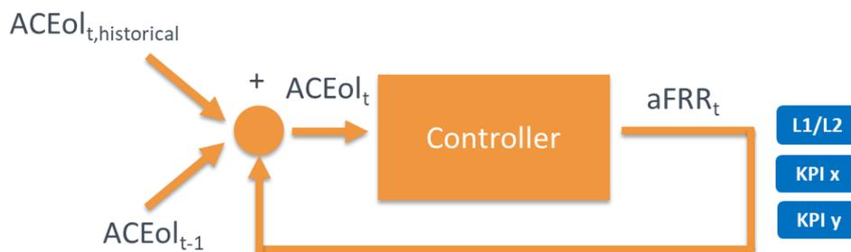
Figure 19: Visual representation of the LFC controller
