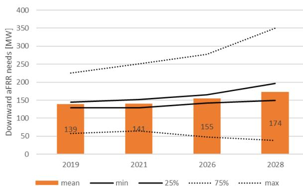
Average, min / max and 25% - 75% percentiles of the upward (left) and downward (right) aFRR needs towards 2028 for the worst case
