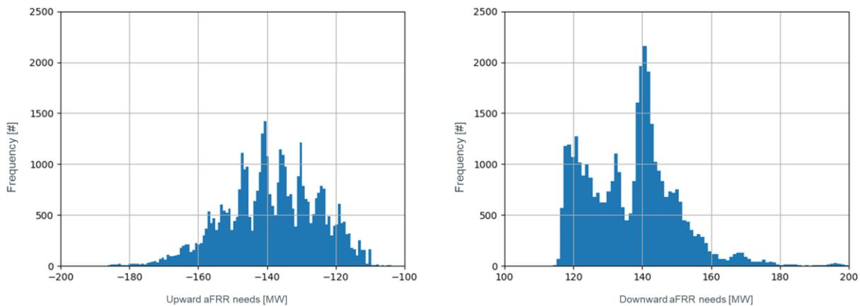
Figure 38: Distribution of the upward (left) and downward (right) aFRR needs over the test set
