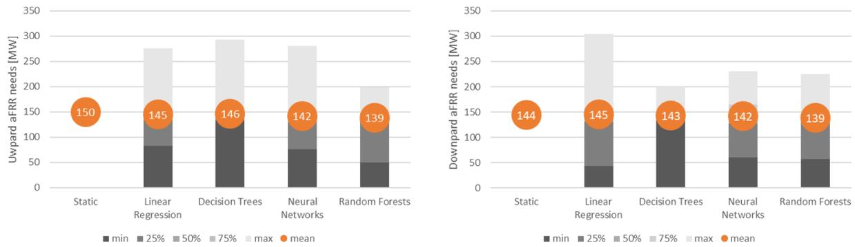
Figure 37: mean, min, max and 25, 50, 75% percentile for the upward (left) and downward (right) aFRR needs for the different algorithms investigated
