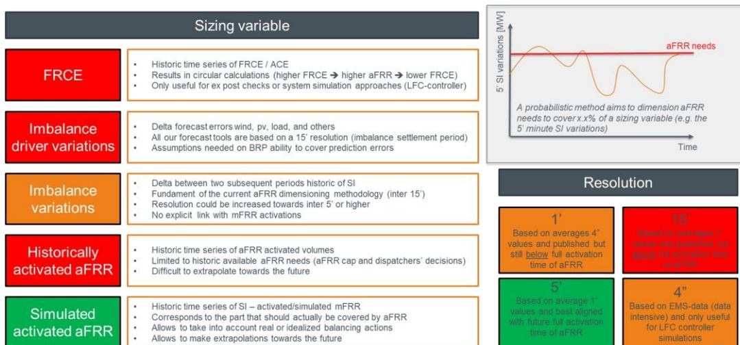
A possibility could be found in simulation methods which can immediately take into account the activation of the dimensioned aFRR. A new method based on emulating Elia's LFC-controller is investigated in Section 3.3 that determines
