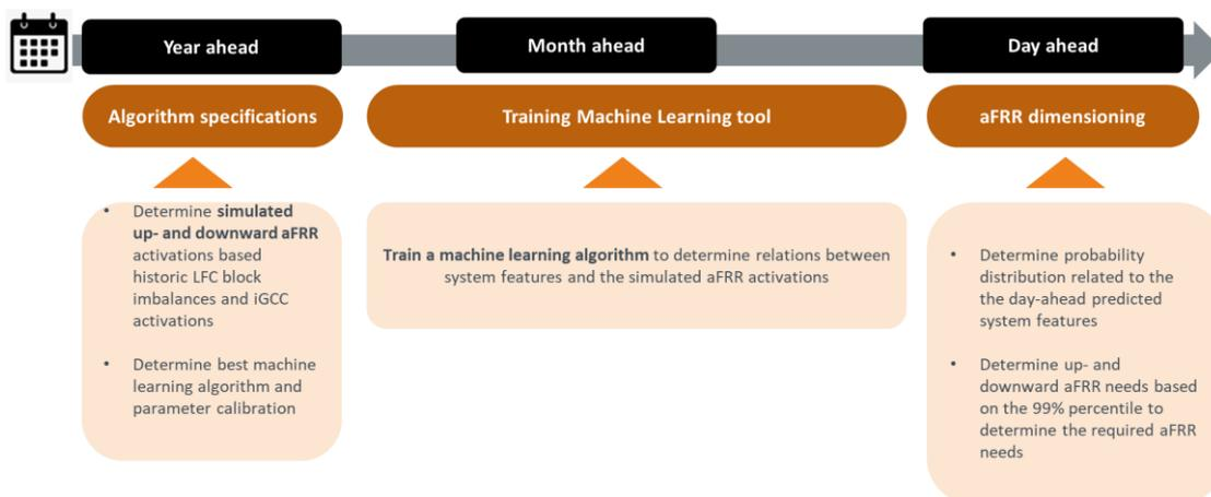
Figure 21: dynamic dimensioning process of aFRR needs
