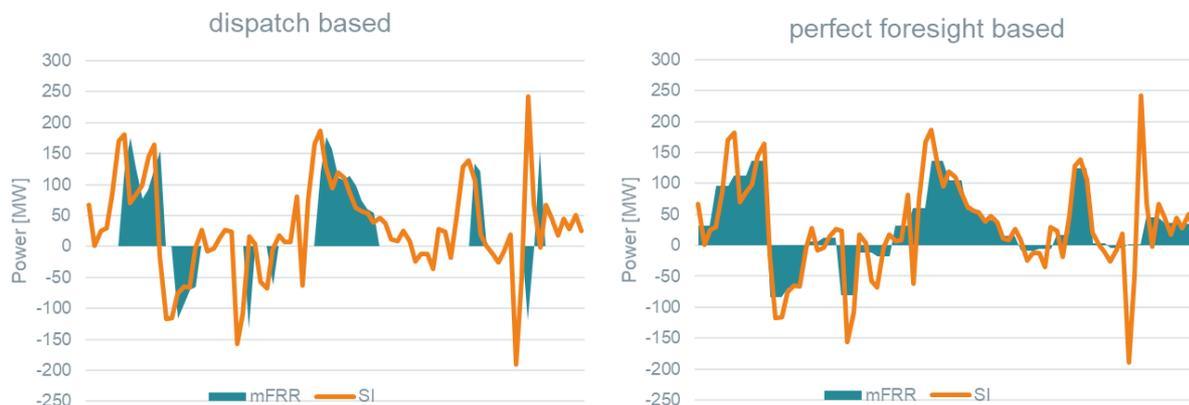
Figure 18: Illustration of simulated mFRR activations in function of the LFC block imbalance
