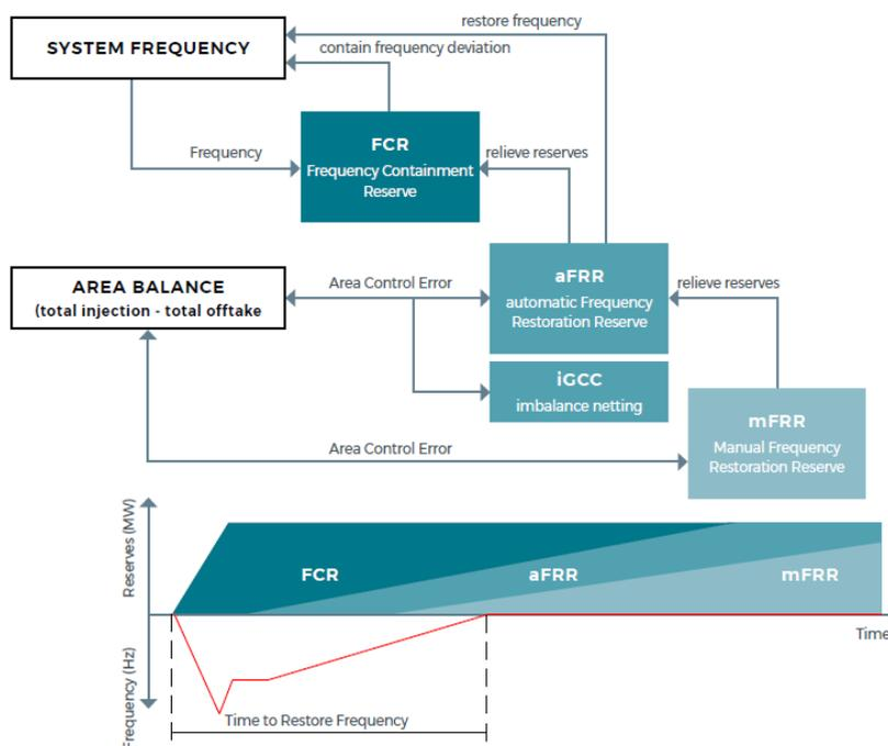
Figure 2: Schematic overview of the activation of operating reserves
