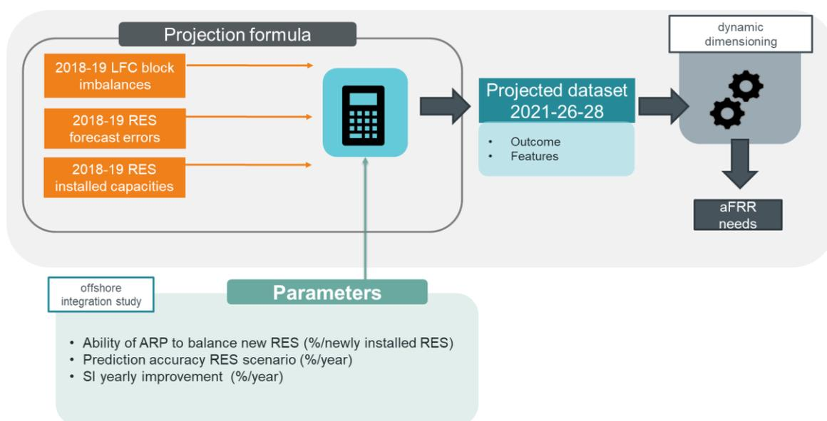
Figure 39: Overview of the methodology for making projections of the aFRR needs towards 2028
