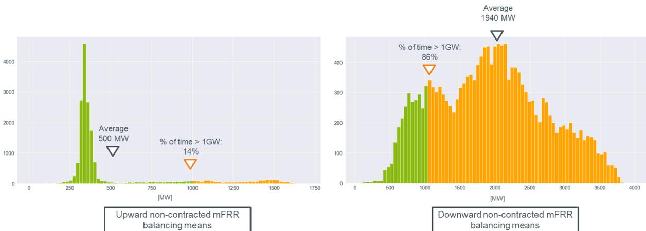
Figure 32: Histogram of available non-contracted mFRR balancing means for upward (left) and downward (right)
