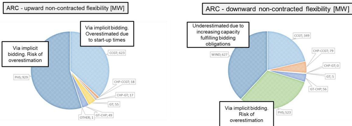
Figure 11: Available regulation capacity (including pumped-hydro storage) per technology in 2020
