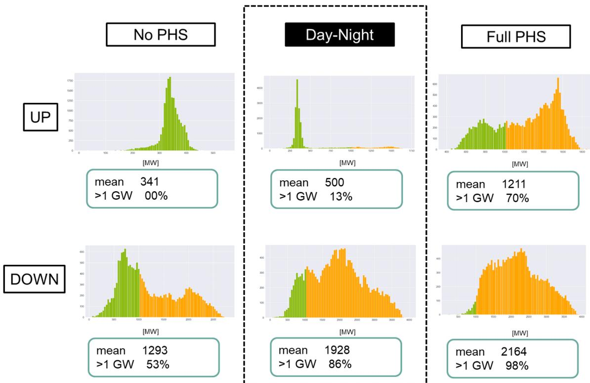
Figure 29: Histograms of available non contracted balancing energy bids for mFRR for sensitivities on pumped-hydro storage operation
