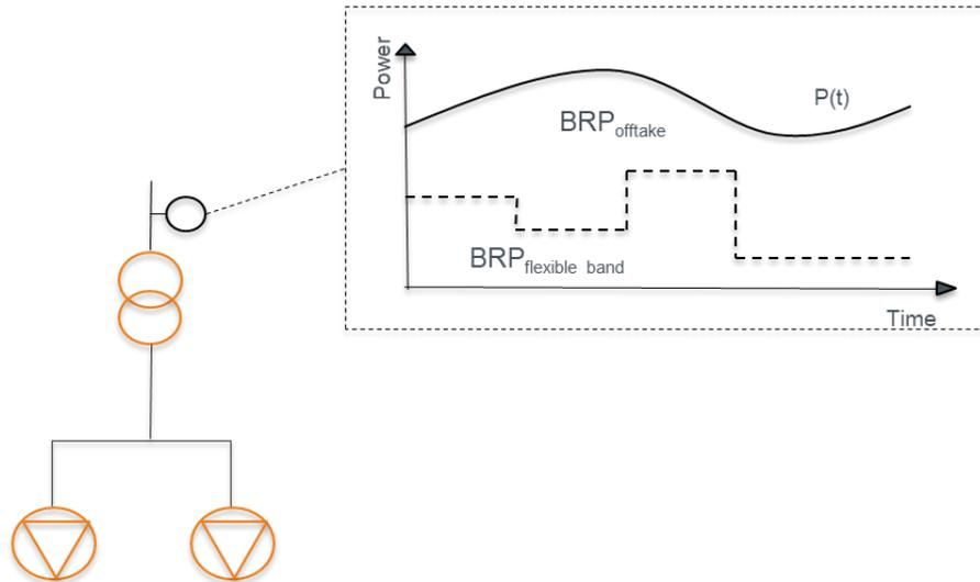
Figure 7: Allocations of energy according to annex 11. The energy is metered at the Access Point level. A changing part of it is allocated to BRP<sub>flexible band</sub> and the rest is allocated to BRP<sub>offtake</sub>.
