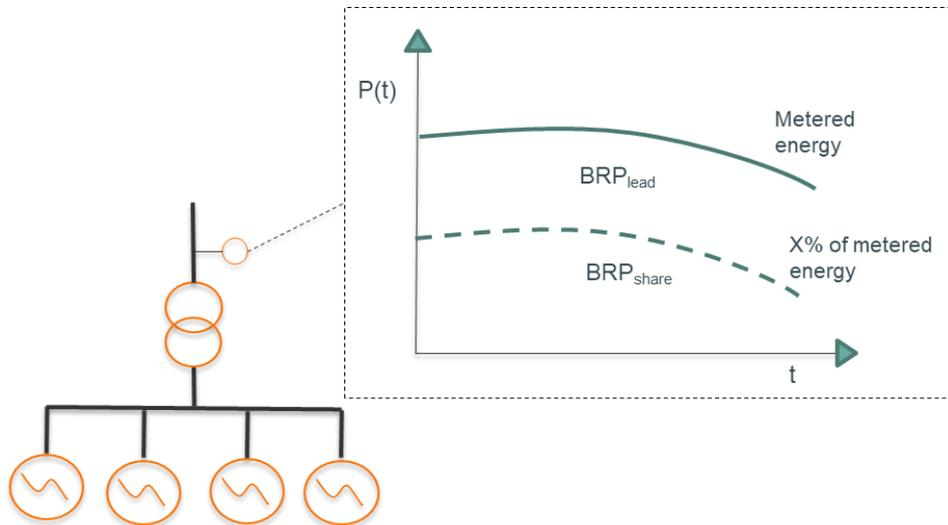
Figure 5: Allocations of energy according to annex 9. The energy is metered at the Access Point and a percentage of it is attributed to different BRPs according to a fixed key.
