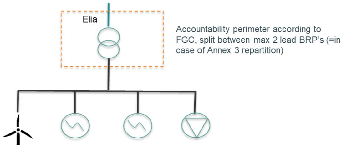
Figure 1: Simple example of a Grid User with several assets behind an Access Point
