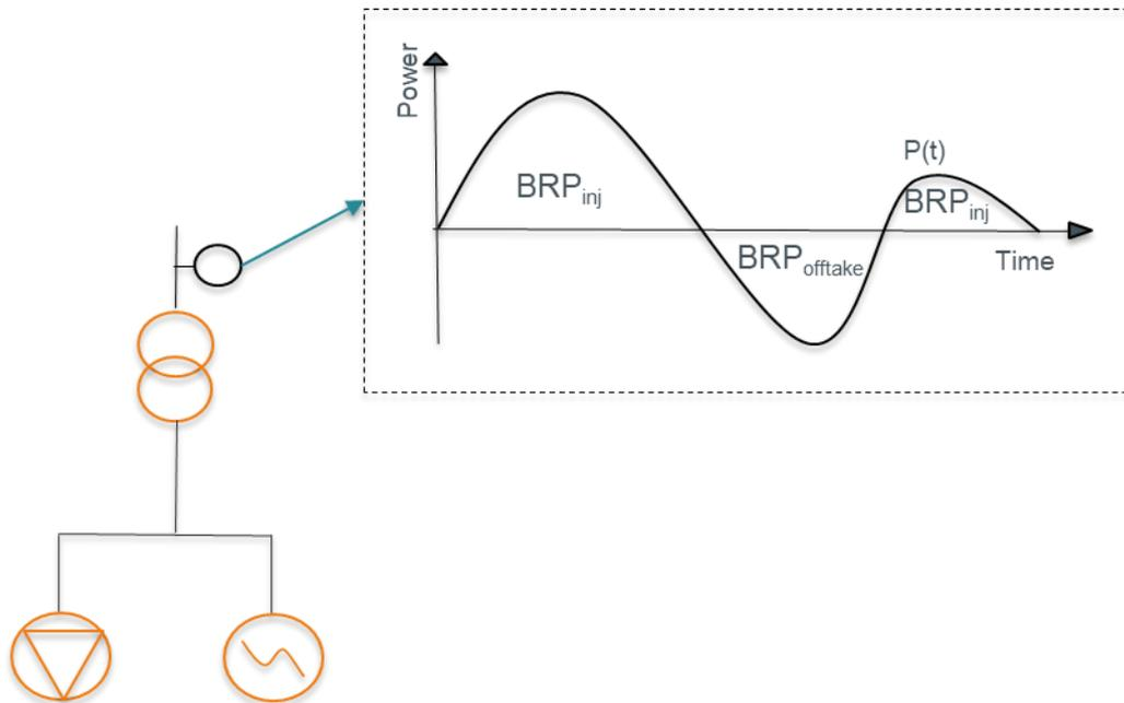
Figure 4: Allocations of energy according to annex 3ter: the BRP responsible for offtake is being attributed the net offtake metered at the Access Point whereas the BRP responsible for injection is being attributed the net injection metered at the Access Point
