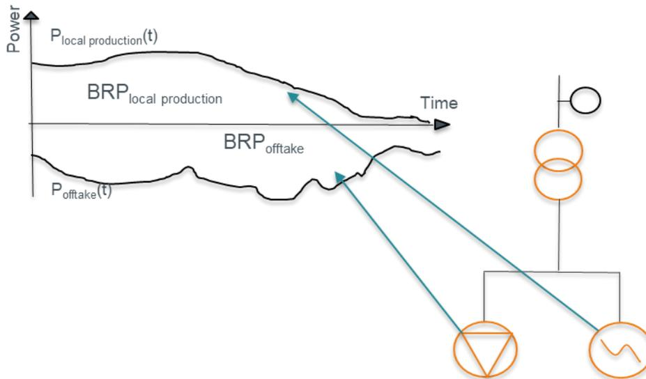
Figure 3: Allocations of energy according to annex 3bis: the BRP responsible for the load is being attributed all offtake metered at asset level whereas the BRP responsible for the local production unit(s) is being attributed all metered volume injected (metered at asset level) by the local production unit(s) (non-netted)
