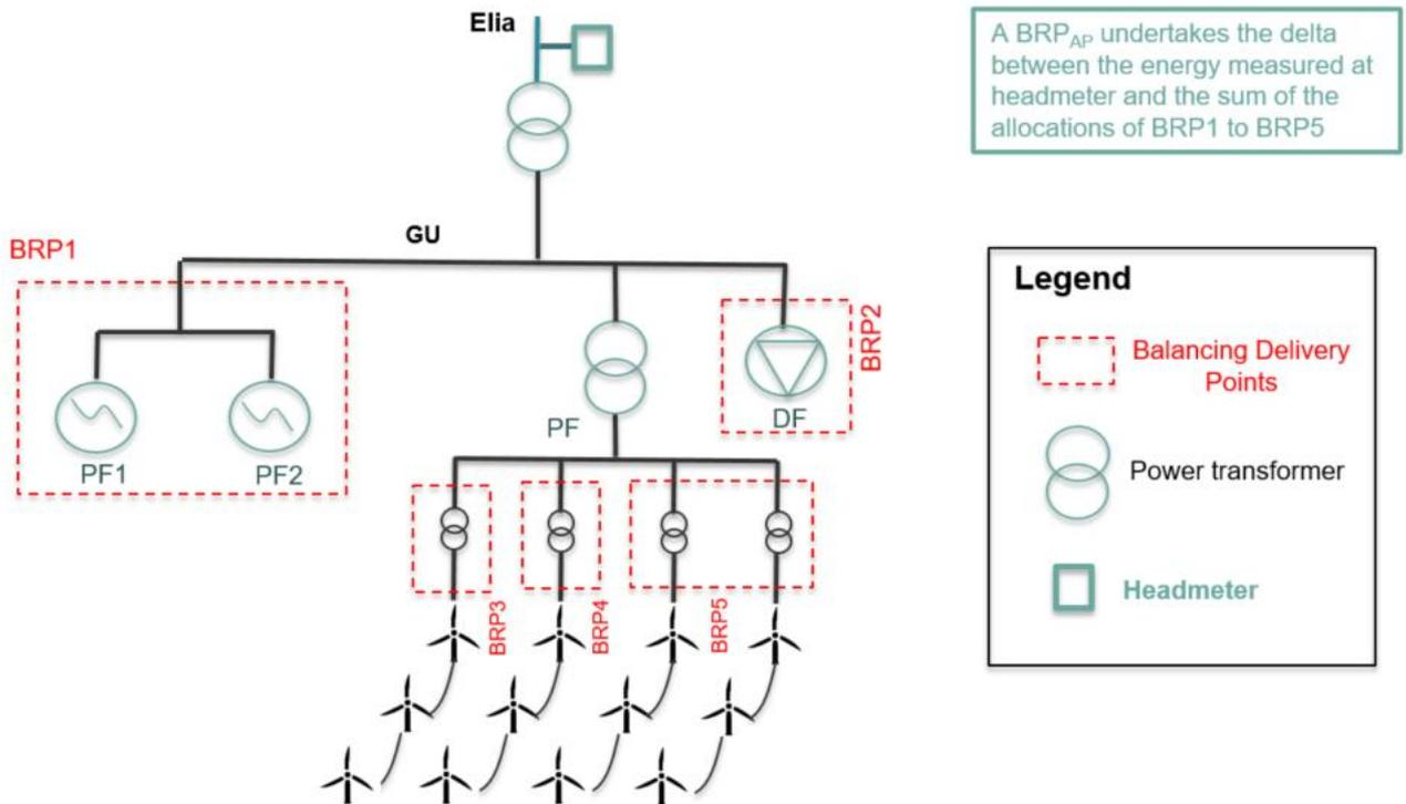
Figure 9: Schematic example of the proposed multi-BRP design. To be noted that for the different strings of wind turbines the anchoring is at metering points, not transformers.
