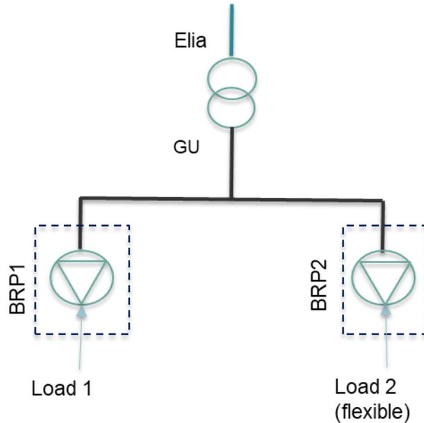
Figure 2: Example of a possible configuration where a separate BRP<sub>source</sub> is designated only for the asset providing flexibility
