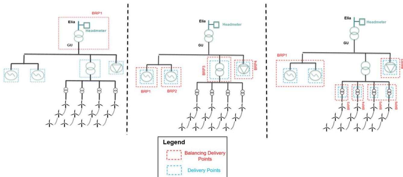
Figure 12: Three different examples of possible configurations of BDPs and DPs
