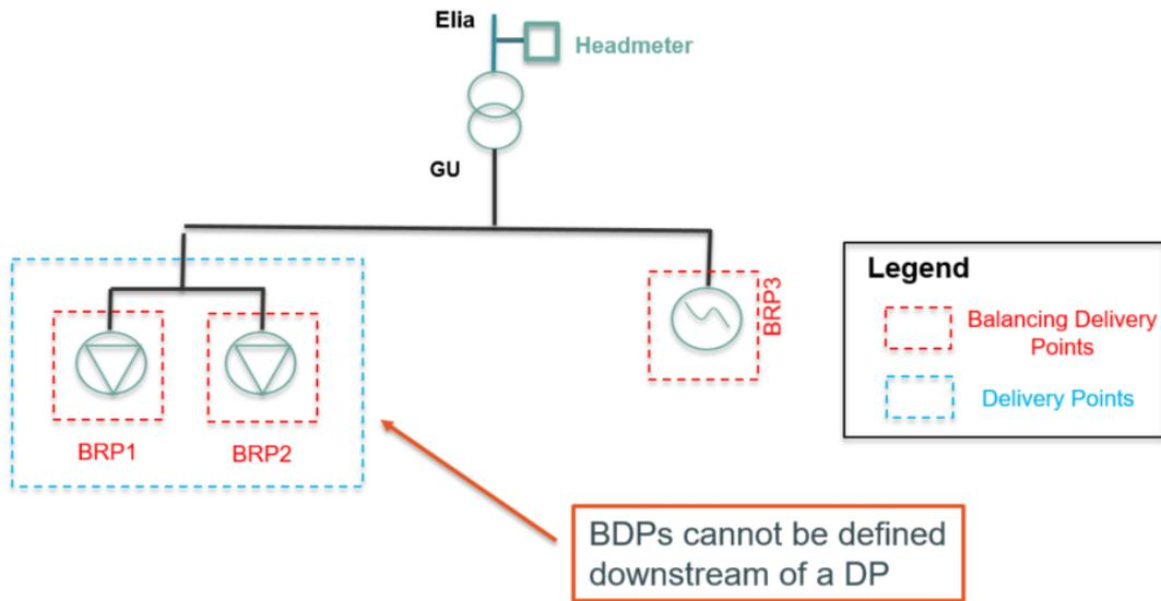
Figure 13: Example of a non-possible configuration of BDPs and DPs
