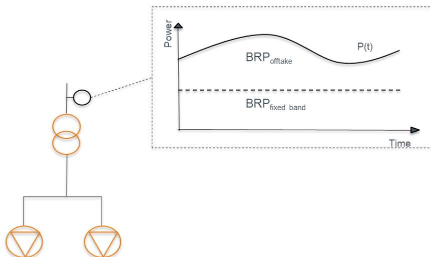
Figure 6: Allocations of energy according to annex 10. Energy is measured at the Access Point. A fixed part of it is allocated to the  $BRP_{fixed\ band}$  and the rest is allocated to the  $BRP_{offtake}$
