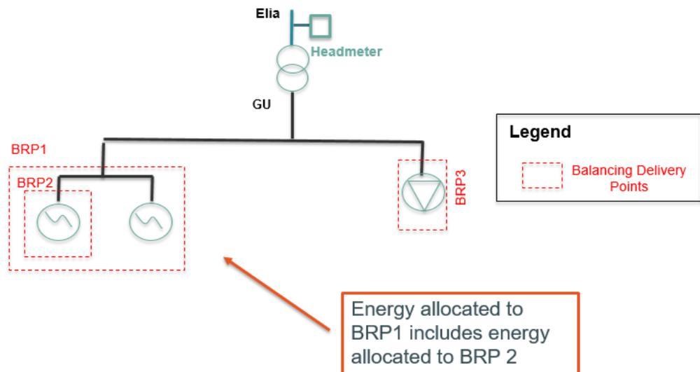
Figure 10: Not allowed configuration due to overlap of BDPs perimeter
