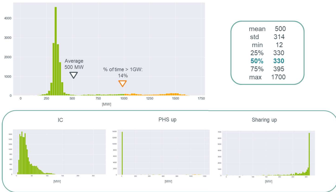
Figure 26: Histogram of predicted available upward non-contracted mFRR balancing energy bids (upper) and breakdown per category (lower)
