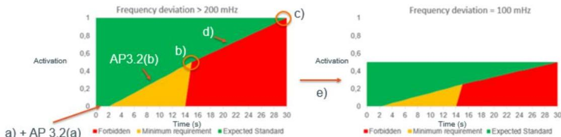
Figure 1: Visual representation of expected FCR activation for a frequency deviation of at least 200 mHz and of 100 mHz
