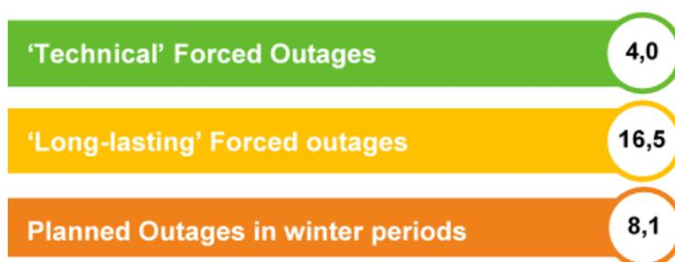
Figure 11: Outage Rates [in %] that could be considered for an equivalent forced outage for nuclear technology
