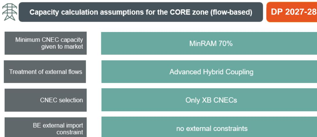
Figure 5: Overview of assumptions for the Core flow based domain creation
