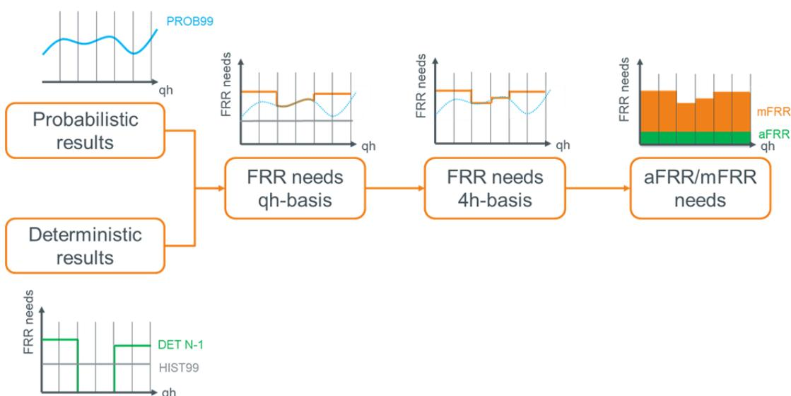
**Figure 3 : Calculation process of the FRR/aFRR/mFRR needs**
