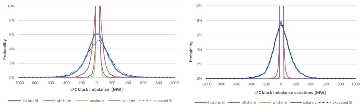
Figure 7: Extrapolation of the LFC block imbalance towards the expected LFC block imbalance (SI) for 2020
