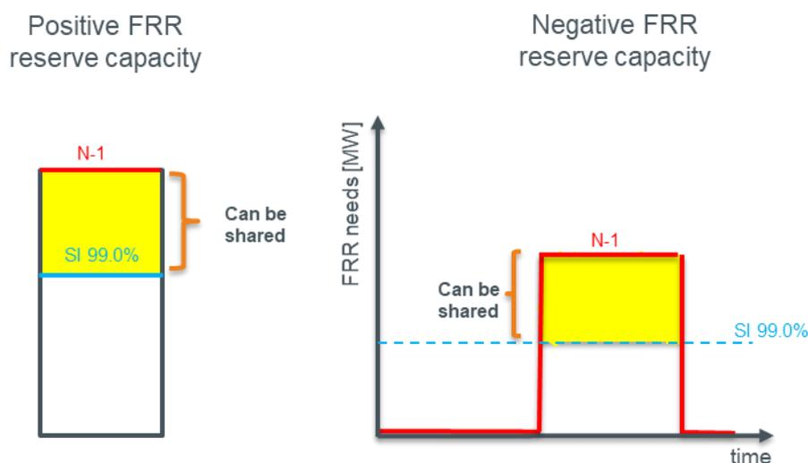
Figure 11: Visual representation of the maximal sharing potential following SOGL by the surface between dimensioning incident (N-1) and historic LFC-block imbalances (SI 99%) for dimensioning positive FRR needs (left) and negative FRR needs (right)
