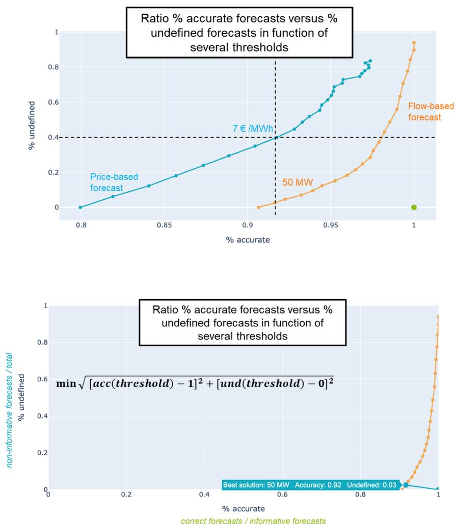
**Figure 6 : ratio accurate / undefined forecasts comparing a price-based and flow-based forecasts for different thresholds (up) and methodology to determine the threshold in view of a multi-objective optimization (lower)**
