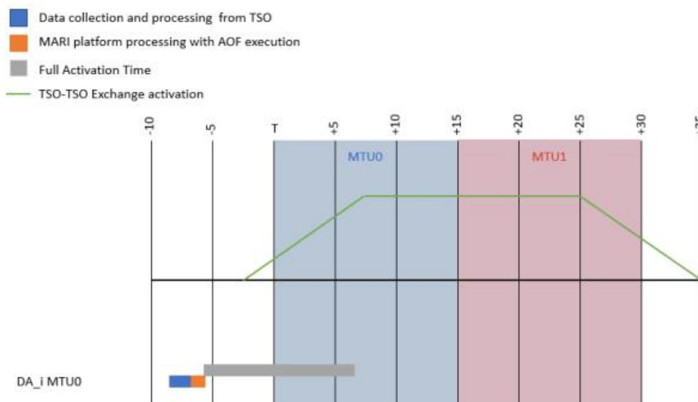
Figure 9 - Timing and activation of a mFRR bid that has been accepted during a Direct Activation process for Market Time Unit MTU0 (extract from the MARI AOF Public Description available on ENTSO-e website)
