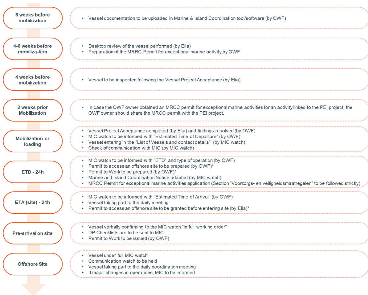
Figure 39 : Flow chart vessel
