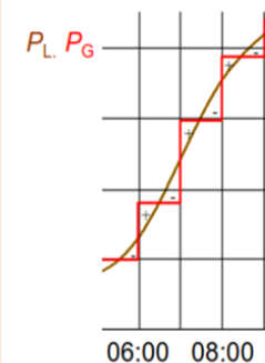
Load and generation difference during a change of Market Time Unit (MTU)
