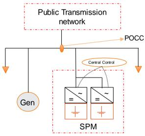
Figure 1 Example of Storage Park Module grid connection
