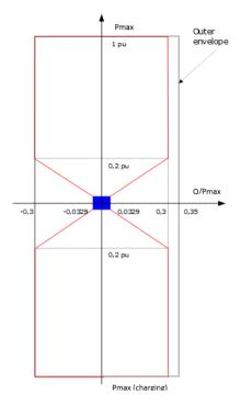
Figure 6: Reactive power capability for a Type C and D SPM.
